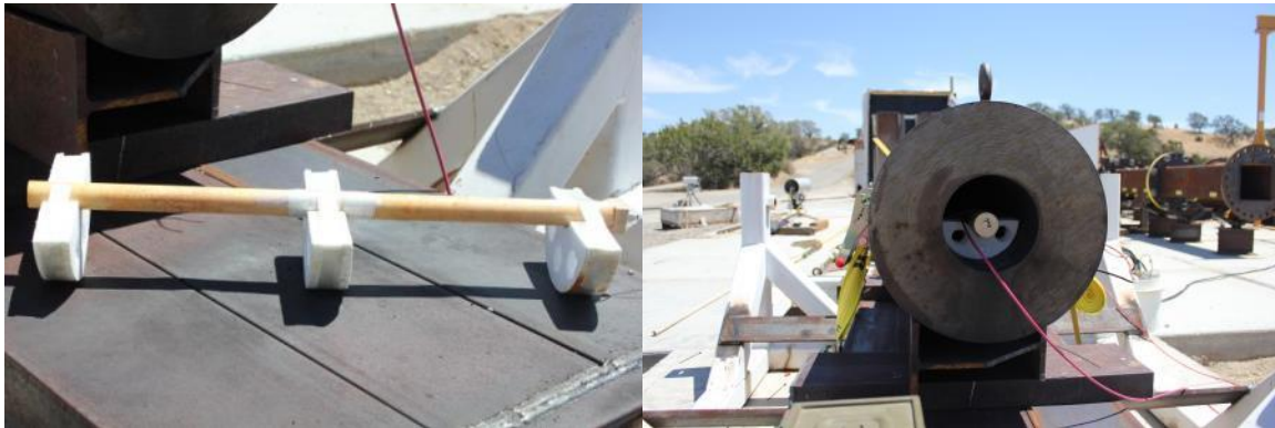
Figure 8. Comp B explosive charge and driver section.
