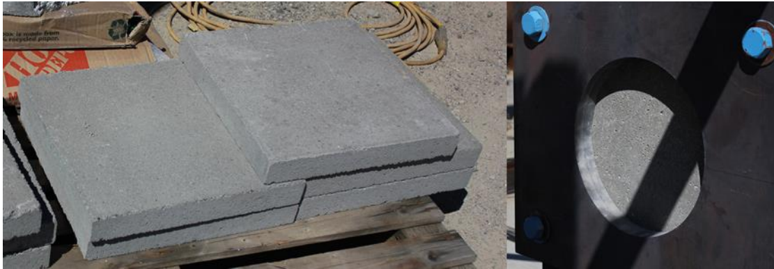
Figure 6. CMU samples before (left) and after (right) being mounted in the supports.
