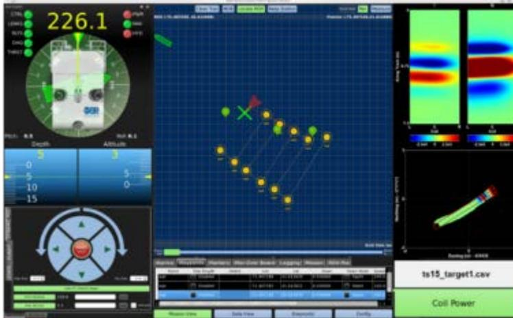
Figure 64. User interface for waypoint mission control. The center portion of the screen illustrates the waypoints input by the user to which the ROV-EM system is commanded to navigate. Multiple waypoints can be entered to configure a multi-point mission plan.
