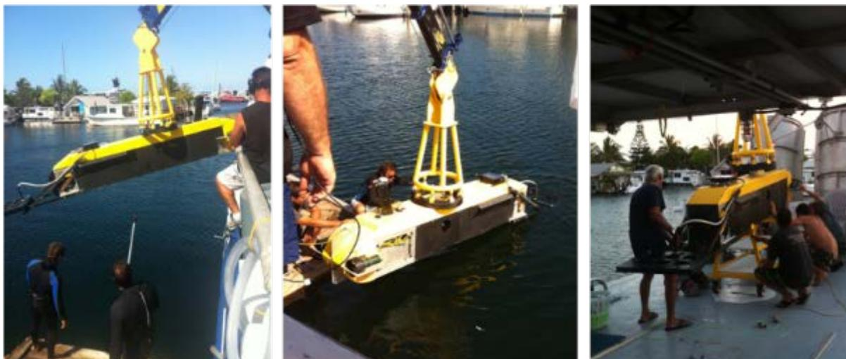
**Figure 71. Dolores HAUV-1000 integrated ROV-EM system launch and recovery operations. The system requires sufficient deck space and hoist capability to deploy over the side of the vessel.**
