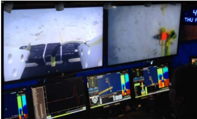
Figure 28. Overall topside operator interface. The two top monitors display real-time imagery from the forward-looking camera image with MFDA array in view (right-side) and downward-looking camera view with UXO in view. The bottom monitors display (from left to right) profile data of select MFDA data channels, openSEA workspace views with different system parameters shown.
