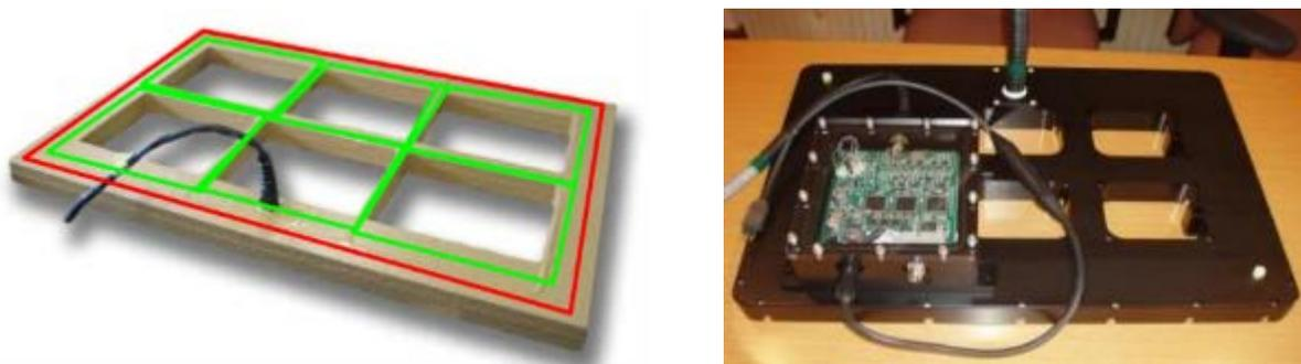
**Figure 2 Left: Photograph of the original equipment manufacturer MFDA EMI sensor head with a single transmitter coil (red) encompassing three differential receivers (green). The receivers are configured as oppositely wound figure-8 shaped pairs to cancel the primary field from the transmitter. Right: Photograph of the MFDA EMI sensor array and electronics encased in pressure vessels for marine operations.**
