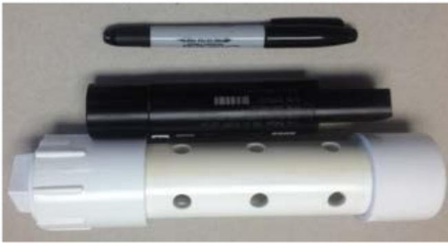
Figure 51. Photograph of the Onset HOBO environmental monitoring device used to sample background water column conductivity and temperature during ROV-EM tests.
