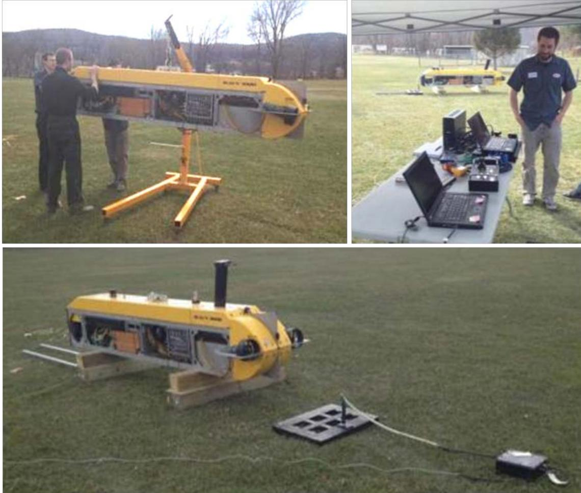
**Figure 6. Photographs of the dry-land noise test set up and configuration.**
