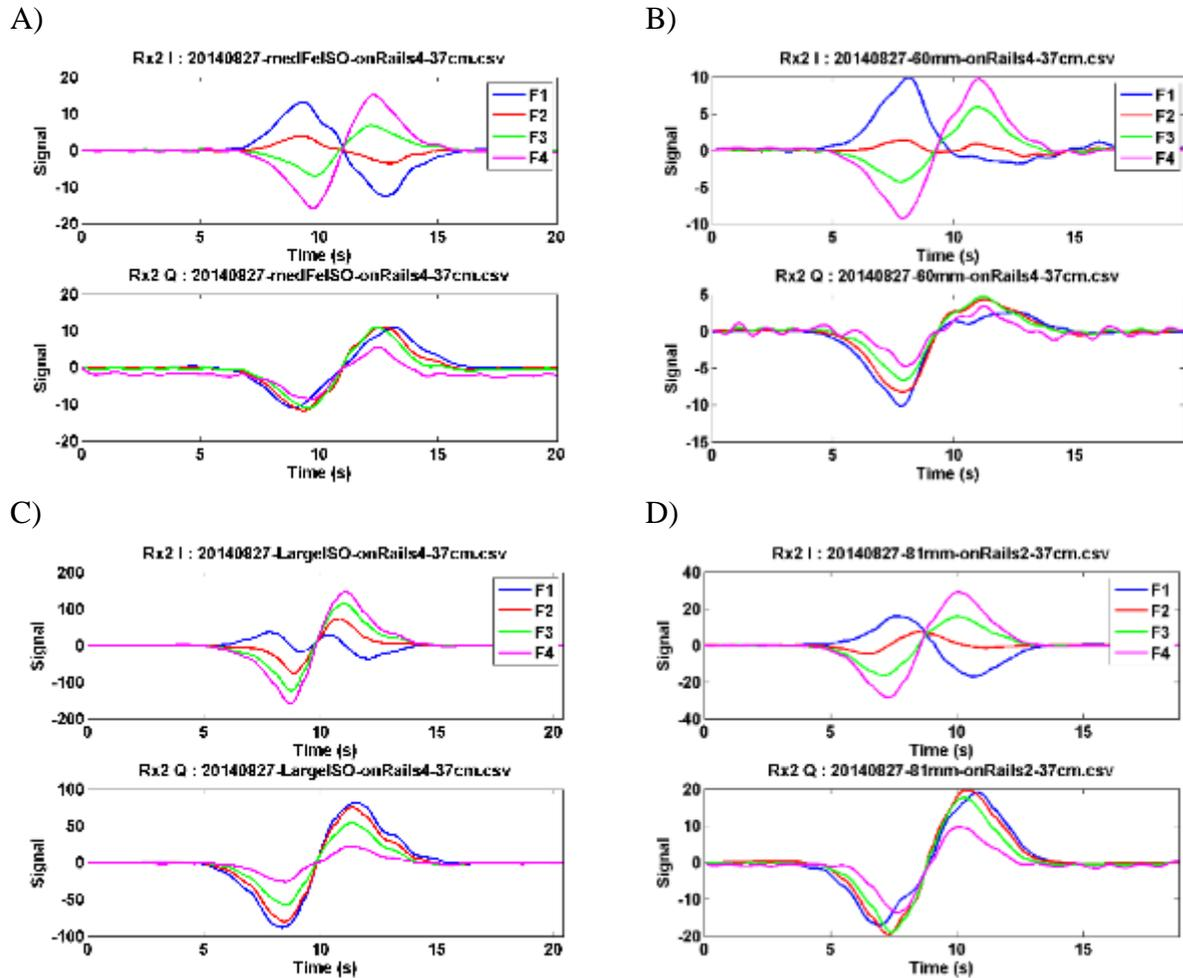
**Figure 18. Time series profiles of various targets pulled under the array during in-water testing: A) Medium ISO, B) 60mm UXO, C) Large ISO, and D) 81mm UXO. The top plot for each set of target profiles represents the in-phase signals for the four frequencies recorded in the center receiver channel and the bottom plots represent the quad-phase signals.**
