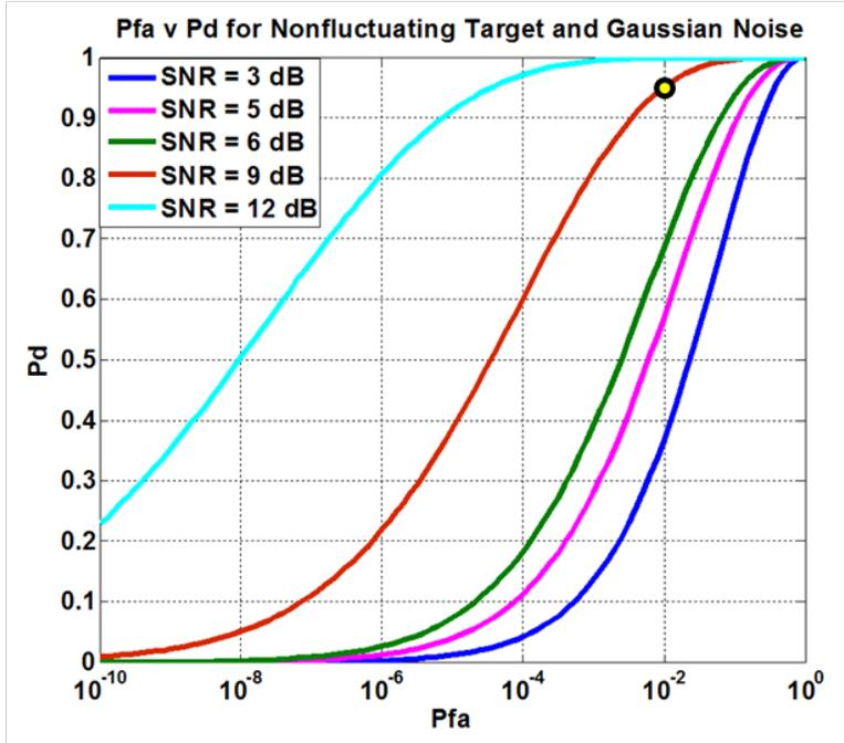
Figure 13. Theoretical ROC curves (in terms of Pd versus Pfa) for SNRs of 3, 5, 6, 9 and 12 dB. Note that our revised success criteria of 95% Pd and 9 dB SNR corresponds to a Pfa of approximately 0.01 as indicated by the yellow dot.
