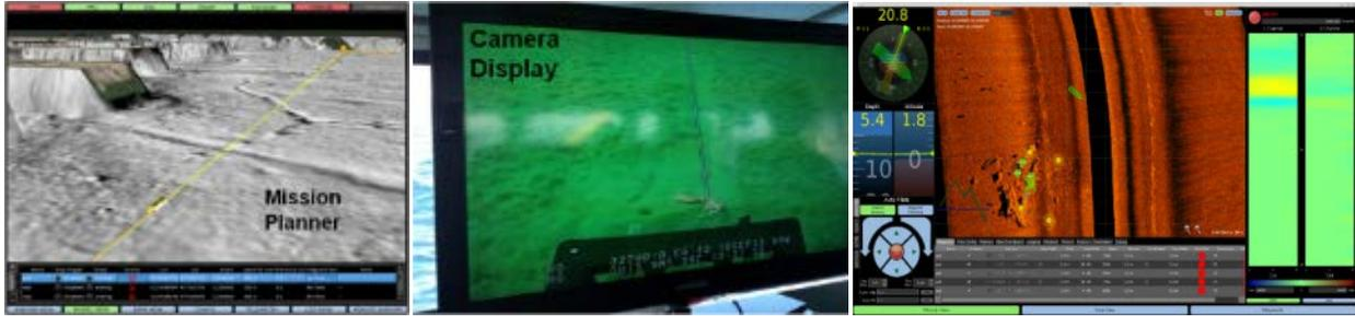
Figure 27. Examples of the topside user interface. Left-to-right: Screenshot of the mission planning GUI used for the NCS, photograph of the camera display screen focused just forward of the EMI Array, and the integrated NCS and MFDA GUI showing ROV system parameters (left panel), mission control profiles (center panel: here waypoint mission plan), and EMI array data maps (right panel).
