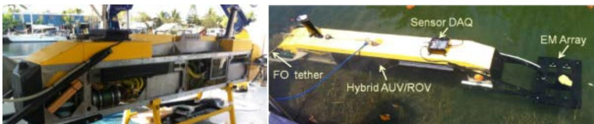
Figure 22. Dolores with the side panel removed (left) and in water with the EM array mounted in the front and EM data acquisition pressure vessel mounted to the top (right).
