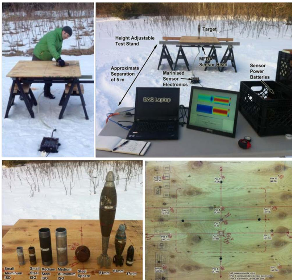
Figure 11. Photographs of the experimental test stand for dry characterization tests.
