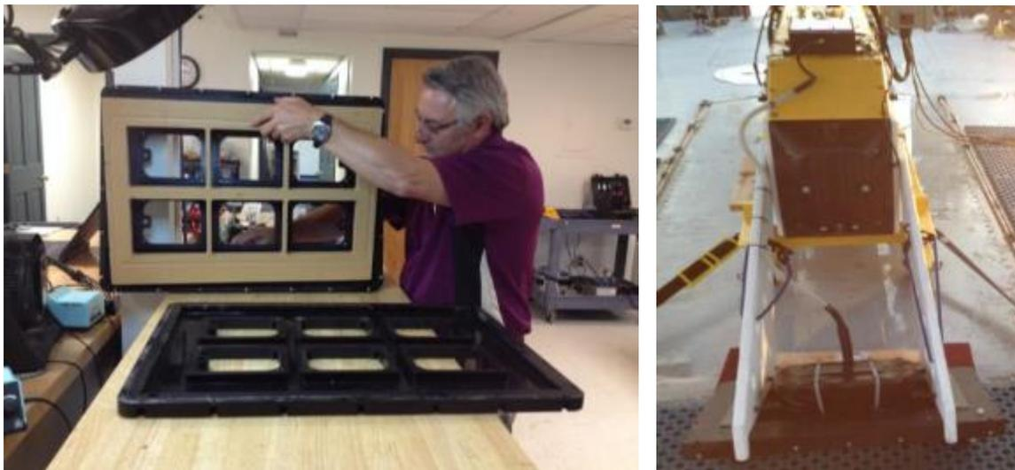
**Figure 3. Left: The MFDA array and marinized enclosure during servicing. Right: The configuration of the MFDA as installed on the HAUV. The MFDA sensor head is rigidly attached to specially fabricated solid PVC arms via fiberglass L-brackets. A ballast was added for trimming the system (aka, the "meatloaf"). It consisted of densely-packed pure silicon glass micro-beads flooded with seawater and sealed in a plastic container.**
