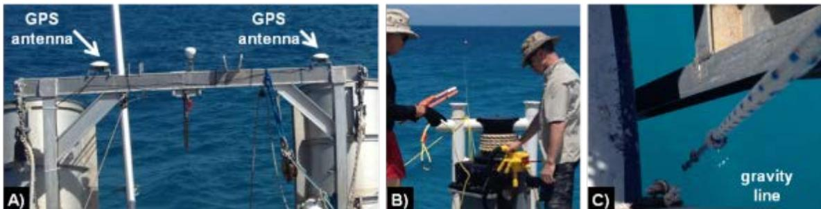
**Figure 47. Photographs of the global positioning survey method for surveying in the grid corners and spar buoy locations. A) Trimble SPS dual antenna GPS system on the abaft beam, B) winch system for used for**
