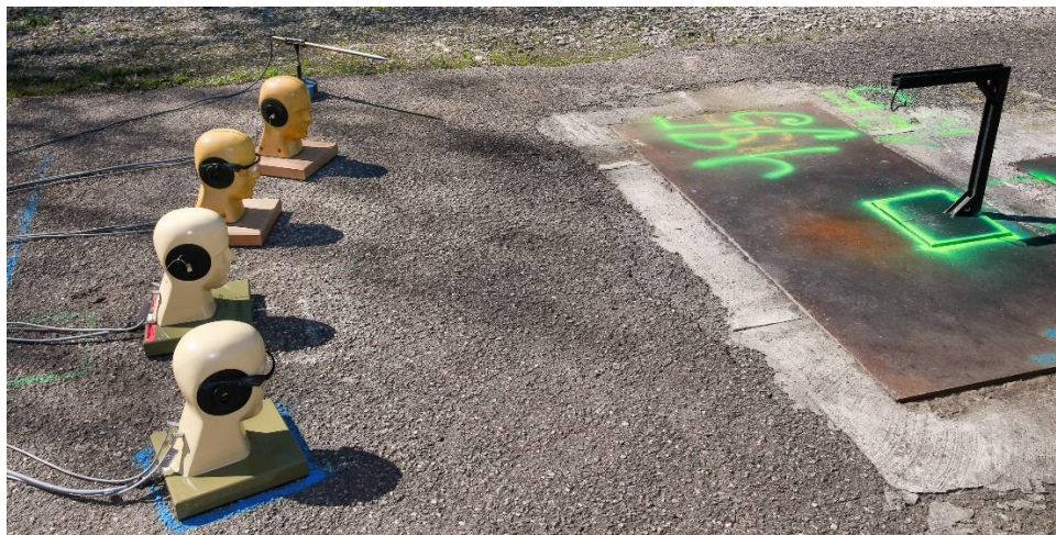
Figure 11. Placement of ATFs and free-field pressure transducer
