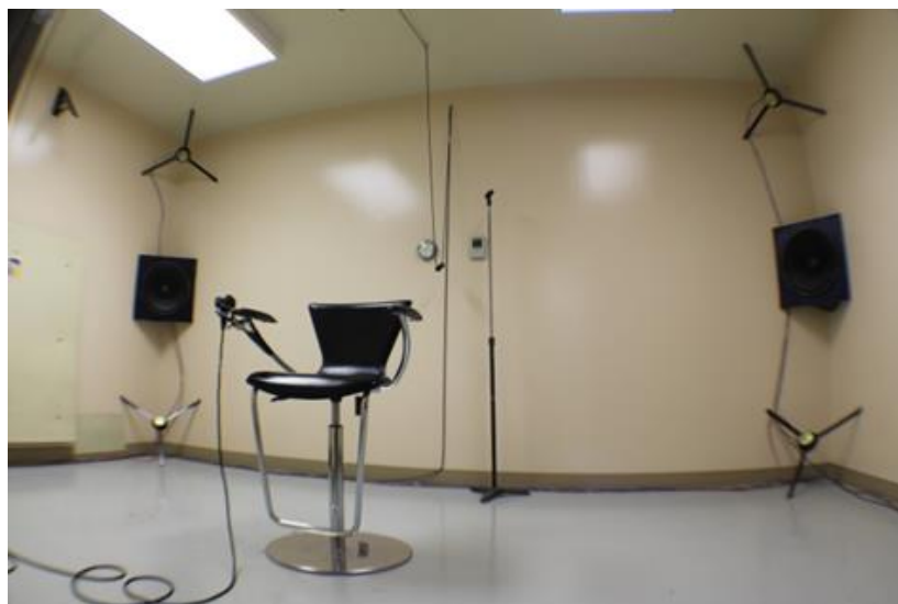
Figure 5. Facility used for measurement of continuous noise attenuation
