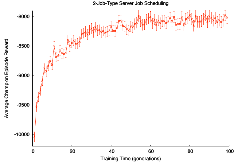
Figure 3.8: This graph shows that NEAT can successfully learn the 2-job-type SJS task. The x-axis shows the training time in generations. In each generation, the agent evaluates 50 policies for 5 episodes, resulting in 250 episodes per generation. Error bars show the standard deviation of the champion performance per generation, averaged over ten learning curves.
