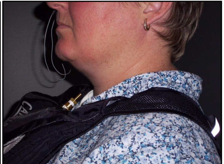
Figure 12. Placement of air vest and correct distance of nozzle from larynx.
