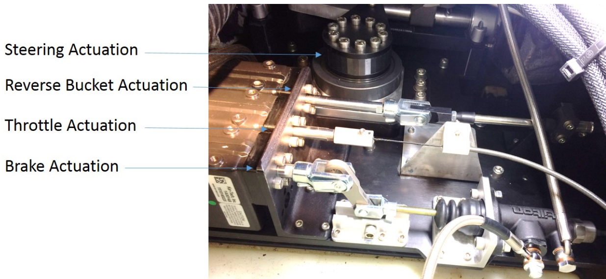
Figure 8. Drive-by-wire actuators.
