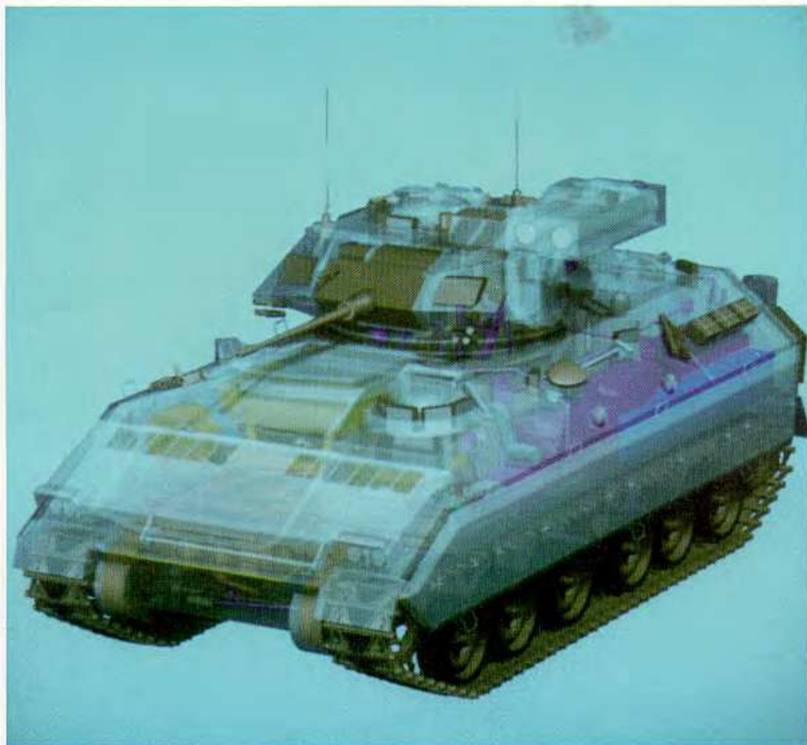
Figure 7. Transparent rendering of the Bradley Armored Fighting Vehicle. Using the same target description file as in Figs. 5 and 6, a lighting model option allows armor to be rendered transparent, revealing internal component placement. ( Geometric model by K. Applin, BRL. )
