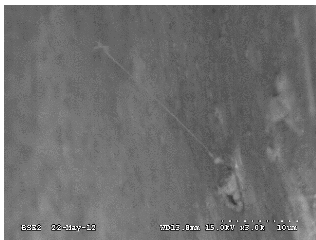
Figure 235: Thin whisker observed on SOT3 termination during second inspection after 4,398 h LTHH, U10, lead 3, 3,000x.
