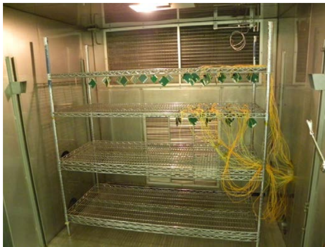
Figure 76: Typical view of test vehicles installed in an environmental chamber.
