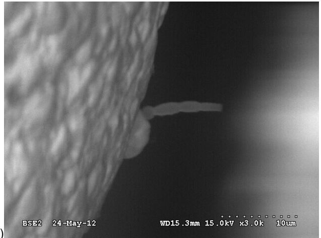
Figure 244: SEM images of whiskers observed during the second inspection on Cu lead frame TQFP64 part termination with a 0-1 contamination level from the second inspection after 4,398 h LTHH; (A) 100x, (B) 400x, (C) left whisker 2,000x, and (D) right whisker, 2,000x (A-QFP-LT-0-1-ncc-2, QFP64, U9, lead 10).
