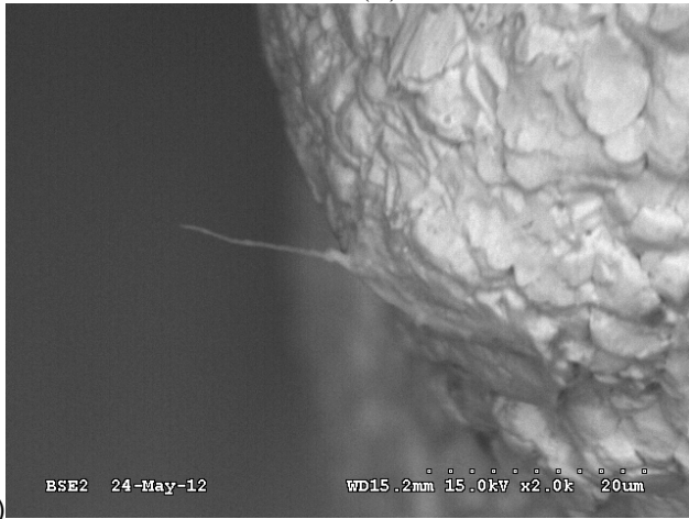
Figure 244: SEM images of whiskers observed during the second inspection on Cu lead frame TQFP64 part termination with a 0-1 contamination level from the second inspection after 4,398 h LTHH; (A) 100x, (B) 400x, (C) left whisker 2,000x, and (D) right whisker, 2,000x (A-QFP-LT-0-1-ncc-2, QFP64, U9, lead 10).
