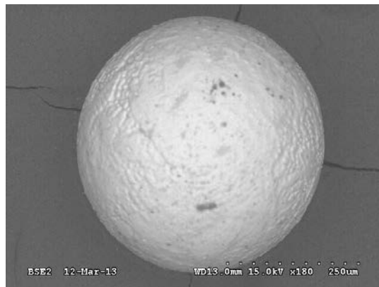
Figure 185: No whisker growth was observed on SAC105 alloy balls soldered with SAC305 solder after 4,000 h of 85°C/85%RH.
