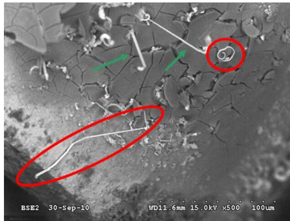
Figure 55: Assembly whisker images (A, C, E) after 500 h, and (B, D, F) 1,500 h at 85°C/85%RH. Circled whiskers appeared after 500 h and did not continue growing after additional 1,000 h. New whiskers formed during additional exposure are shown with arrows.
