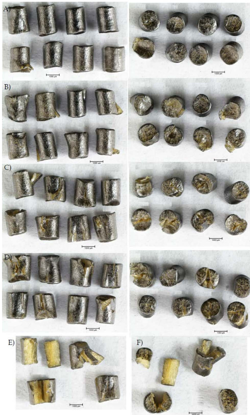
Figure C1.3: Exemplar AR2211 grains compacted at -60^{\circ}\text{C} : A) SA100; B) SA105; C) SA115; D) SA125; E) SA135; and F) SA155 categories.
