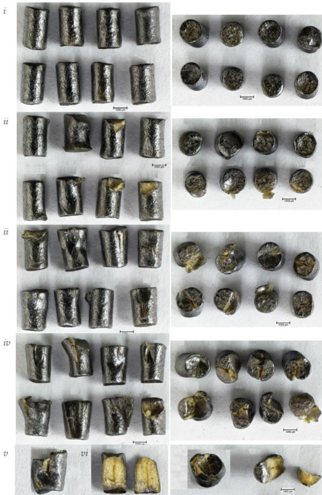
Figure C2.3: Exemplar AR2220 grains post-compaction at a -40^{\circ}\text{C} test condition: i) no visible fracture; ii) web and surface fracture only; iii) fracture up to \frac{1}{4} grain length; iv) fracture up to \frac{1}{2} grain length; v) fracture up to full grain length; and vi) grain shivered.
