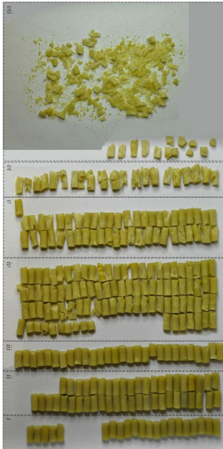
Figure C4.9: BS-NACO, aged for 67 days at 70°C, bed compaction at -60°C: i) no visible fracture; ii) web and surface fracture only; iii) fracture up to \frac{1}{4} grain length; iv) fracture up to \frac{1}{2} grain length; v) fracture up to full grain length; vi) grain shivered; and vii) grain pulverised.
