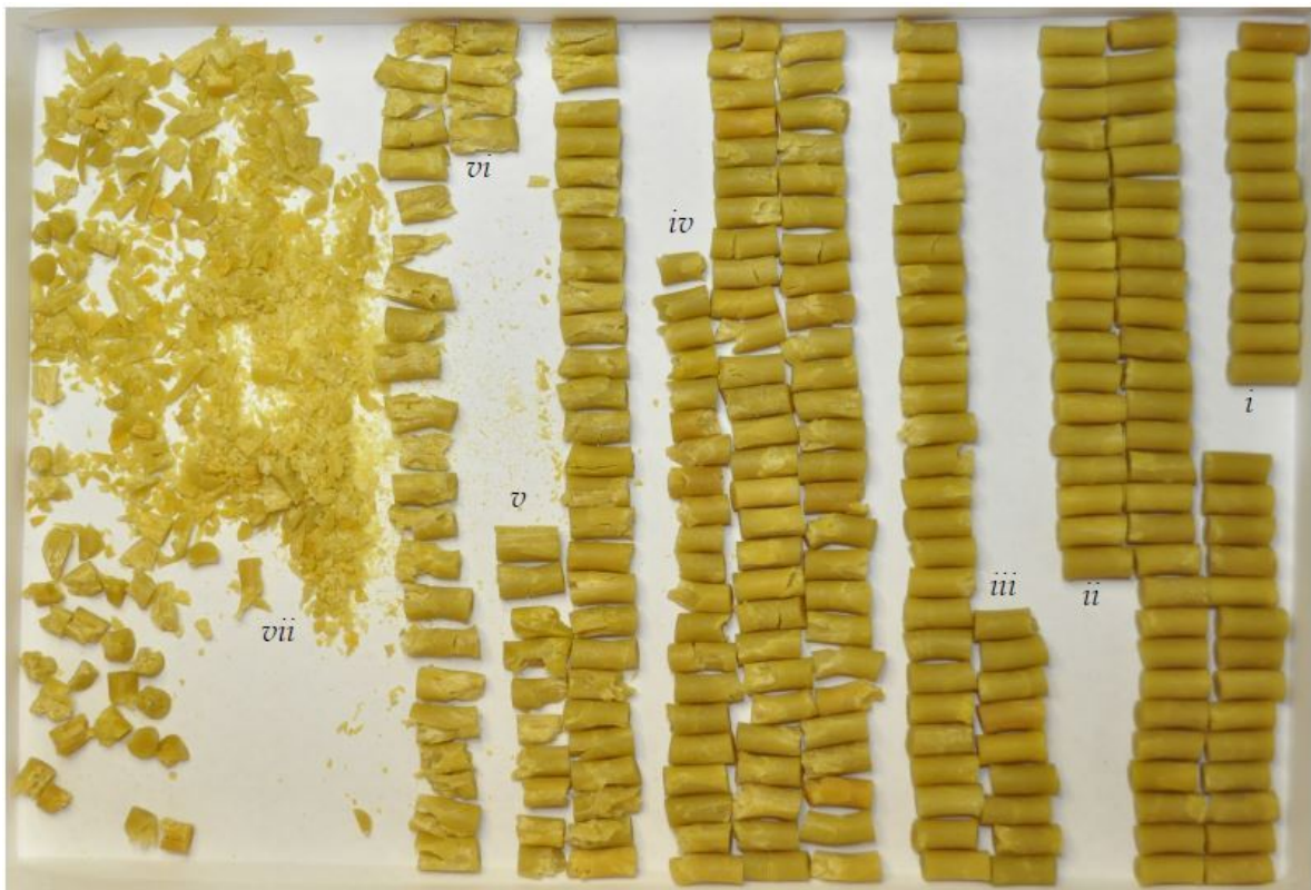
Figure C4.10: BS-NACO, aged for 40 days at 80°C, bed compaction at -60°C: i) no visible fracture; ii) web and surface fracture only; iii) fracture up to \frac{1}{4} grain length; iv) fracture up to \frac{1}{2} grain length; v) fracture up to full grain length; vi) grain shivered; and vii) grain pulverised.
