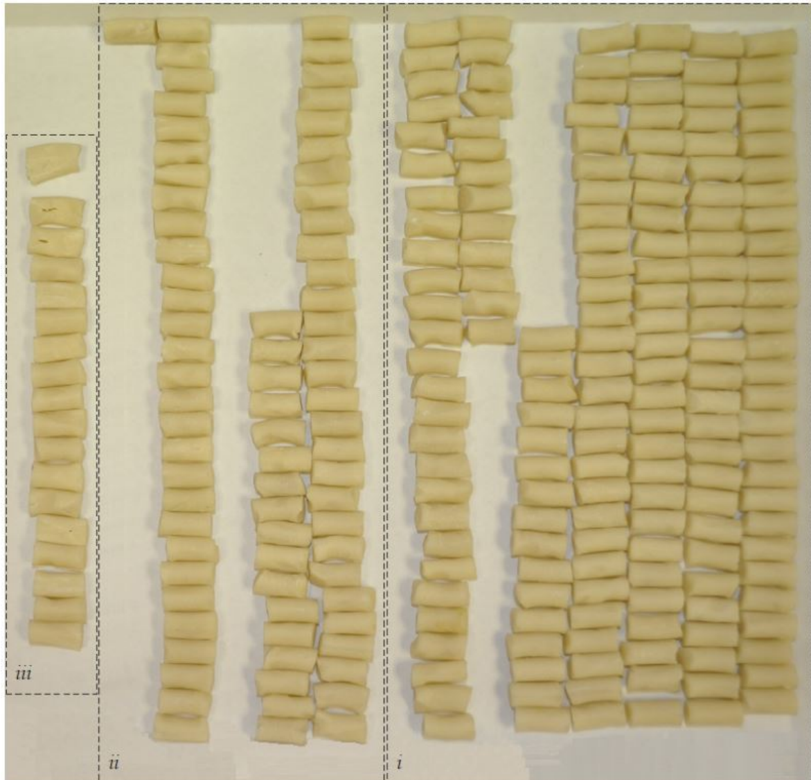
Figure C4.1: BS-NACO bed post-compaction at an ambient temperature test condition: i) no visible fracture; ii) web and surface fracture only; and iii) fracture up to \frac{1}{4} grain length.
