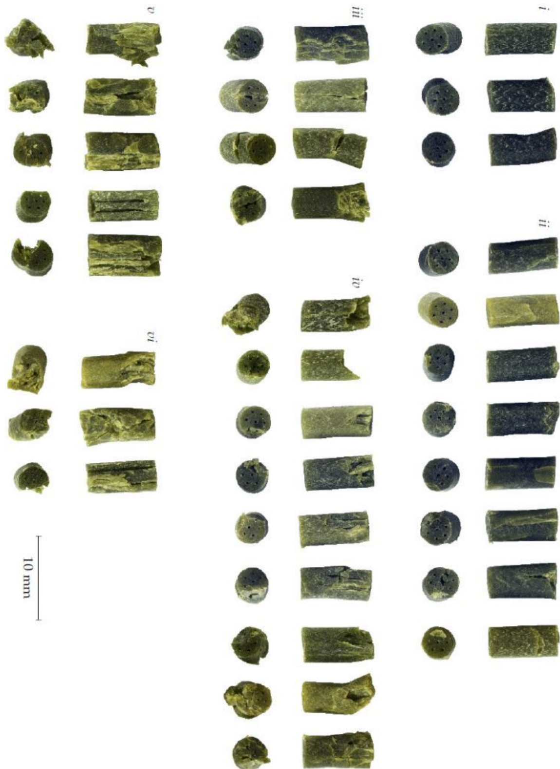
Figure C3.3: Exemplar FNH-025 grains post-compaction at a -40^{\circ}\text{C} test condition: i) no visible fracture; ii) web and surface fracture only; iii) fracture up to \frac{1}{4} grain length; iv) fracture up to \frac{1}{2} grain length; v) fracture up to full grain length; and vi) grains shivered.
