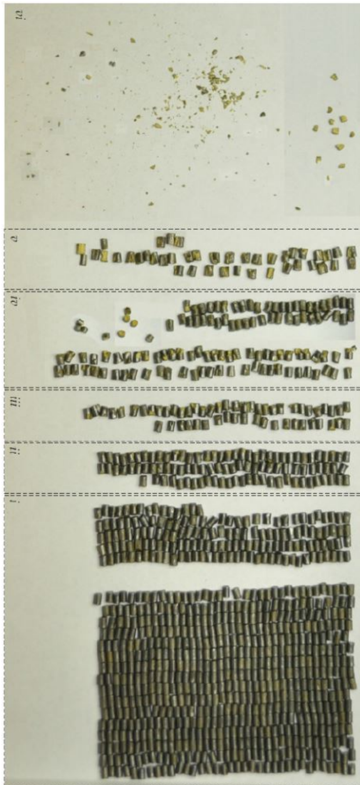
Figure C2.6: AR2220, aged for 42 days at 70°C, bed compaction at -60°C: i) no visible fracture; ii) web and surface fracture only; iii) fracture up to 1/4 grain length; iv) fracture up to 1/2 grain length; v) fracture up to full grain length; and vi) grain pulverised.
