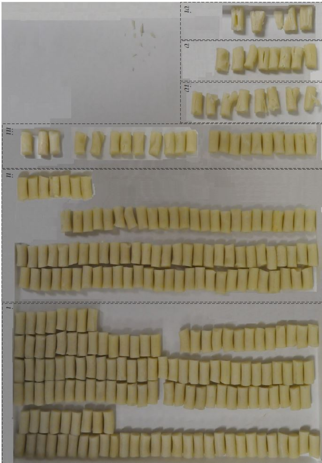
Figure C4.3: BS-NACO bed post-compaction at a -15^{\circ}\text{C} test condition: i) no visible fracture; ii) web and surface fracture only; iii) fracture up to \frac{1}{4} grain length; iv) fracture up to \frac{1}{2} grain length; v) fracture up to full grain length; and vi) grain shivered.
