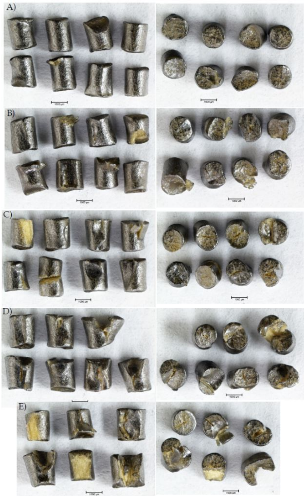
Figure C1.2: Exemplar AR2211 grains compacted at -40^{\circ}\text{C} : A) SA100; B) SA105; C) SA115; D) SA125; and E) SA135 categories.
