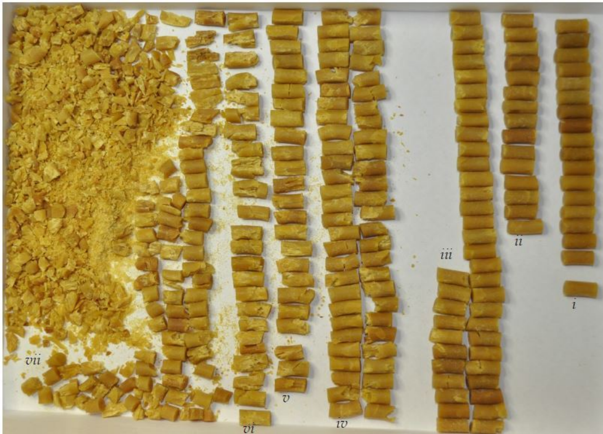
Figure C4.12: BS-NACO, aged for 80 days at 80°C, bed compaction at -60°C: i) no visible fracture; ii) web and surface fracture only; iii) fracture up to \frac{1}{4} grain length; iv) fracture up to \frac{1}{2} grain length; v) fracture up to full grain length; vi) grain shivered; and vii) grain pulverised.
