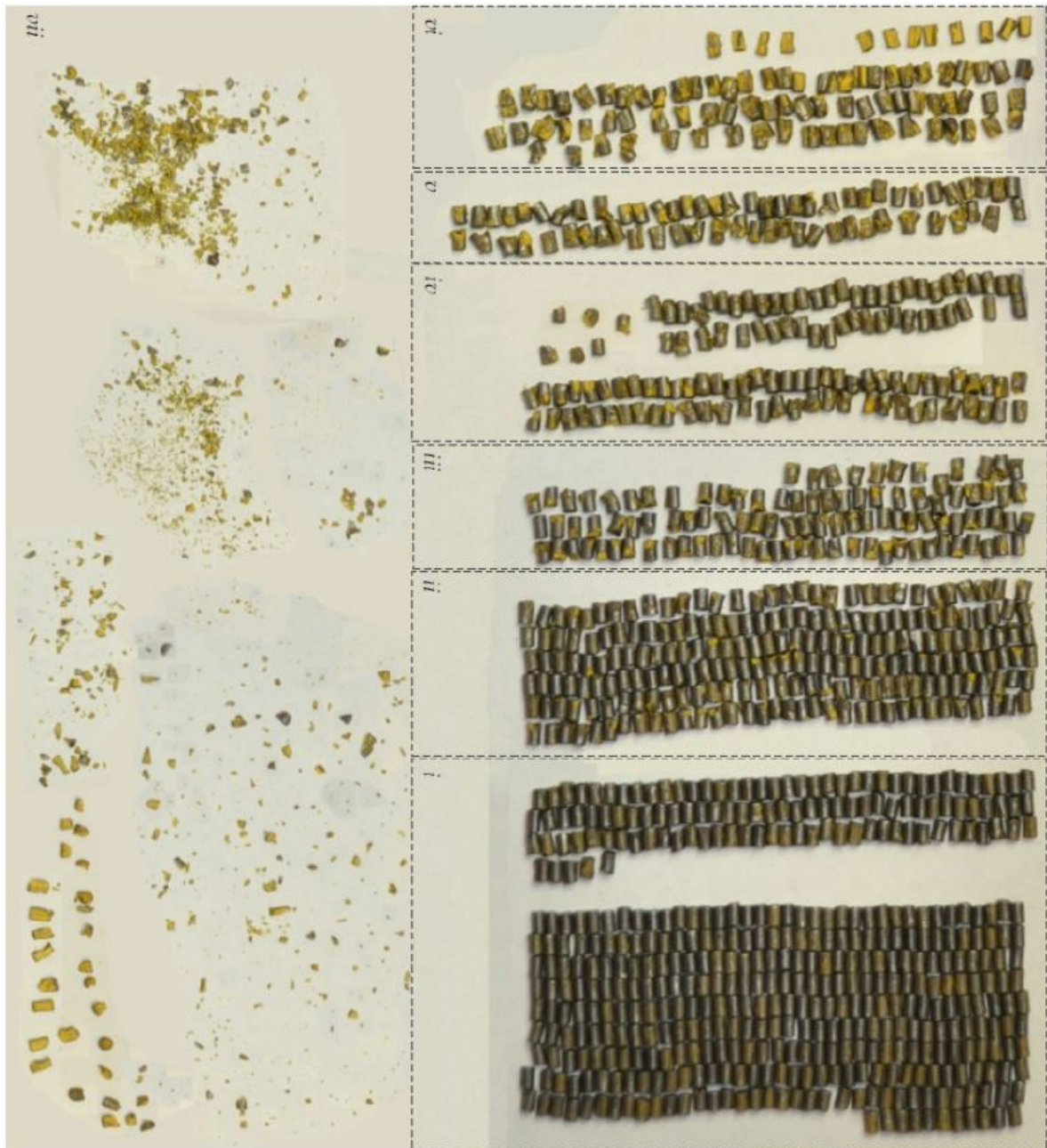
Figure C2.7: AR2220, aged for 86 days at 70°C, bed compaction at -60°C: i) no visible fracture; ii) web and surface fracture only; iii) fracture up to 1/4 grain length; iv) fracture up to 1/2 grain length; v) fracture up to full grain length; vi) grain shivered; and vii) grain pulverised.
