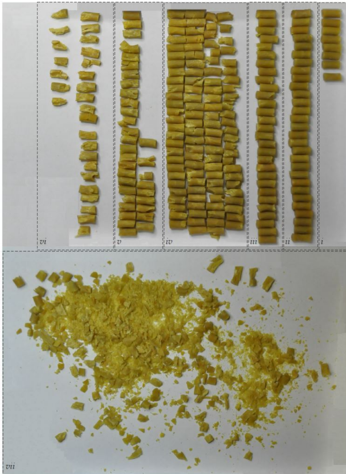
Figure C4.11: BS-NACO, aged for 60 days at 80°C, bed compaction at -60°C: i) no visible fracture; ii) web and surface fracture only; iii) fracture up to \frac{1}{4} grain length; iv) fracture up to \frac{1}{2} grain length; v) fracture up to full grain length; vi) grain shivered; and vii) grain pulverised.
