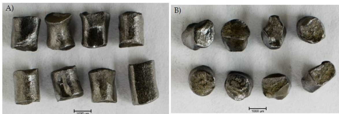
Figure C1.1: AR2211 exemplar grains post-compaction testing at ambient: A) side view; and B) top view.
