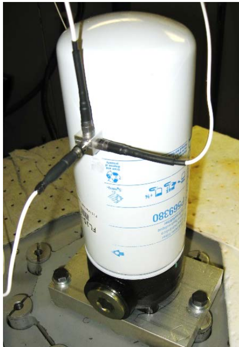
Figure 13. Donaldson, 569380 (FL15-2317) Mounted to Shaker Table
