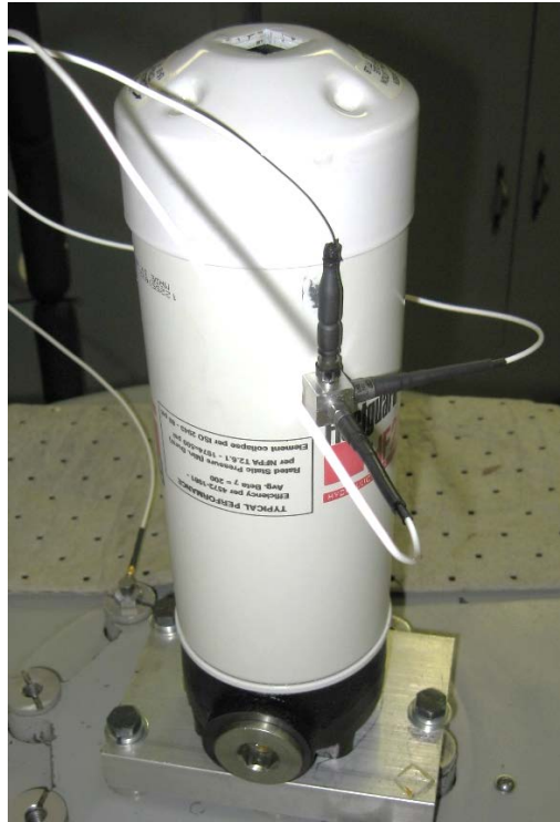
Figure 12. Fleetguard, HF28202 (FL15-2332) Mounted to Shaker Table
