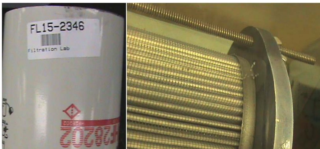
Figure 3. Test Filter Fleetguard, HF28202 (FL15-2346) First Bubble
