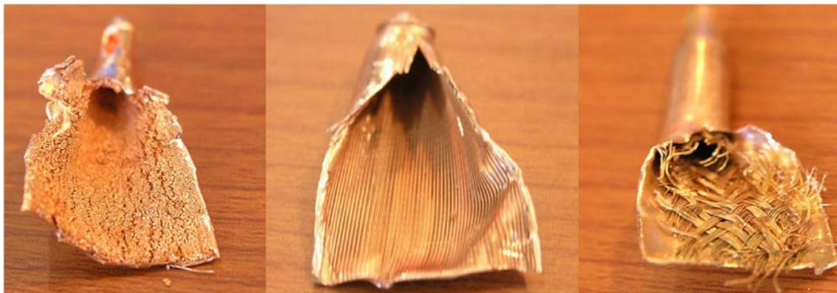
*Figure 2: Different types of wicks; Sintered copper (left), Axial grooves (center), Screen mesh (right)[4]*
