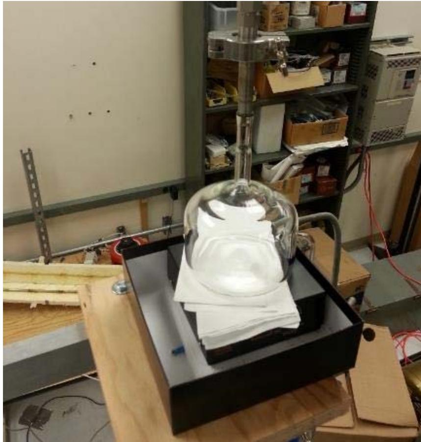
**Figure 82: Degassing chamber and magnetic stirrer**
