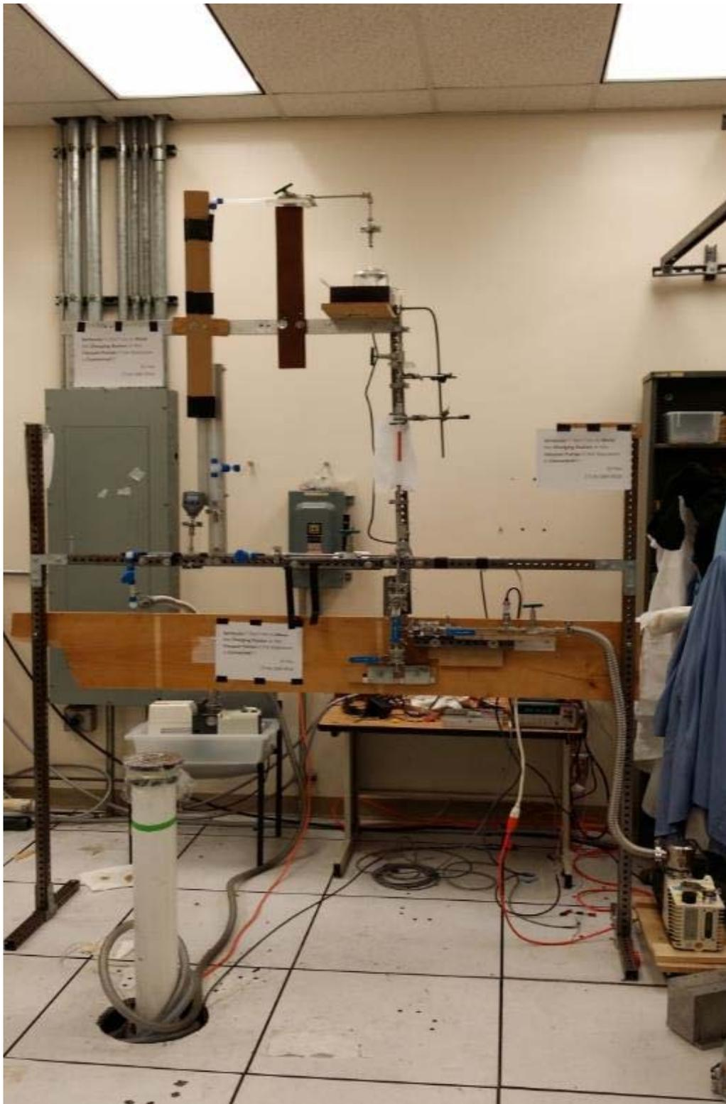
Figure 83: Charging station with degassing feather
