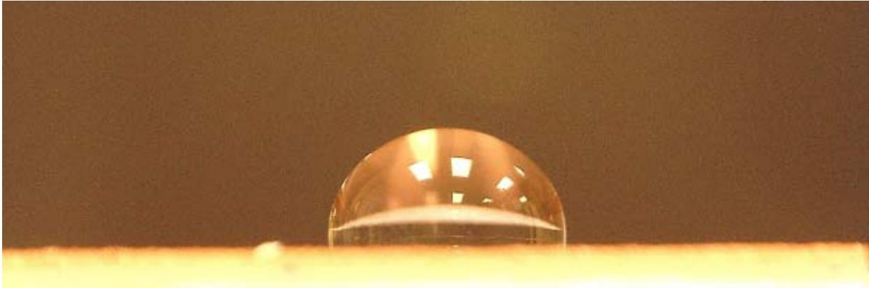
**Figure 46: DI-water on mirror like copper surface**
