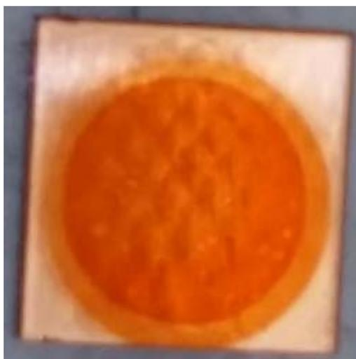
**Figure 30: Copper surface pre-treated by UCLA IAS #1**
