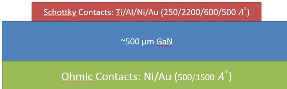
**Fig. 5** Description of device fabrication process
