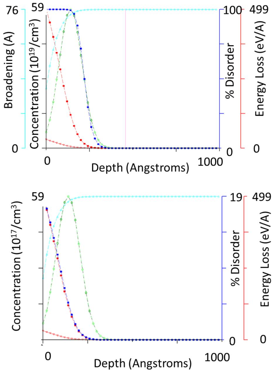
Figure 1. Ion implantation simulations of neodymium in thin films of niobium. Simulations are made at low  $10^{13}\text{cm}^{-2}$  and high  $10^{14}\text{cm}^{-2}$  dose at 60 keV. At high dose, disorder induced is significantly greater and may favor different final arrangement of the ions in the host crystal.
