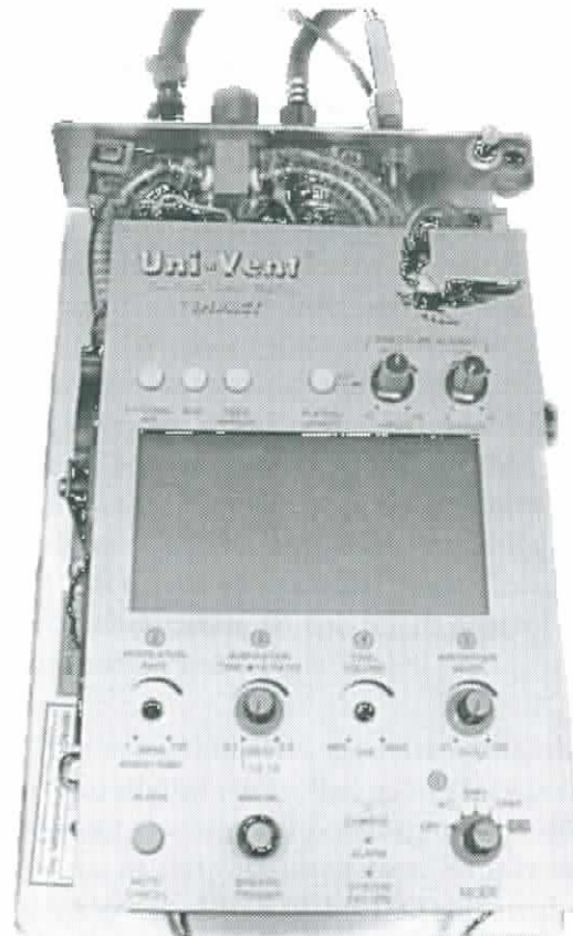
Figure 2.3: The medical ventilator used in this study is a Impact Uni-Vent Model 754. It is a particularly robust ventilator that uses volume settings to specify the ventilation pattern.
