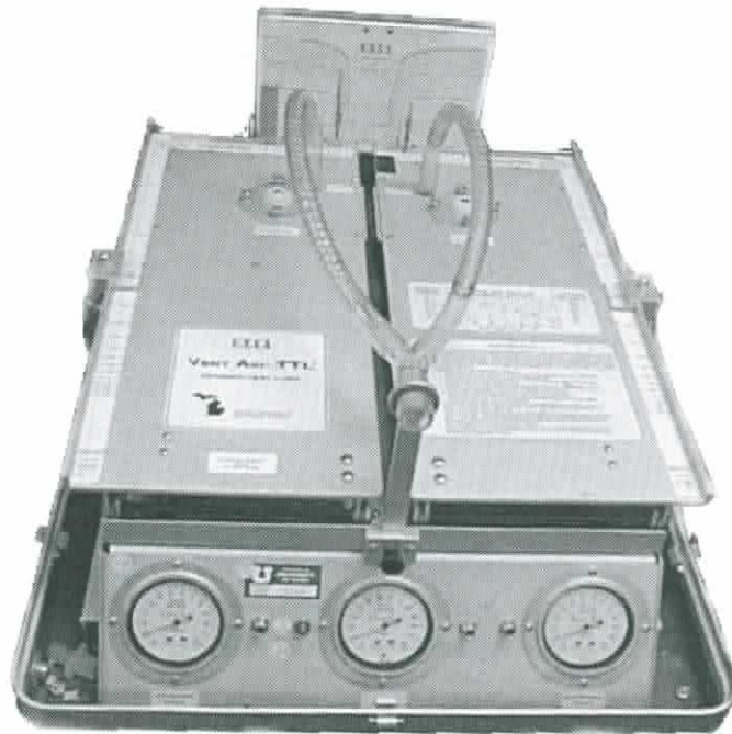
Figure 2.4: This is the mechanical test lung used to test the systems performance. The resistance and compliance can be individually set for each of the two "lungs". This gives a good possibility to simulate different lung pathologies.
