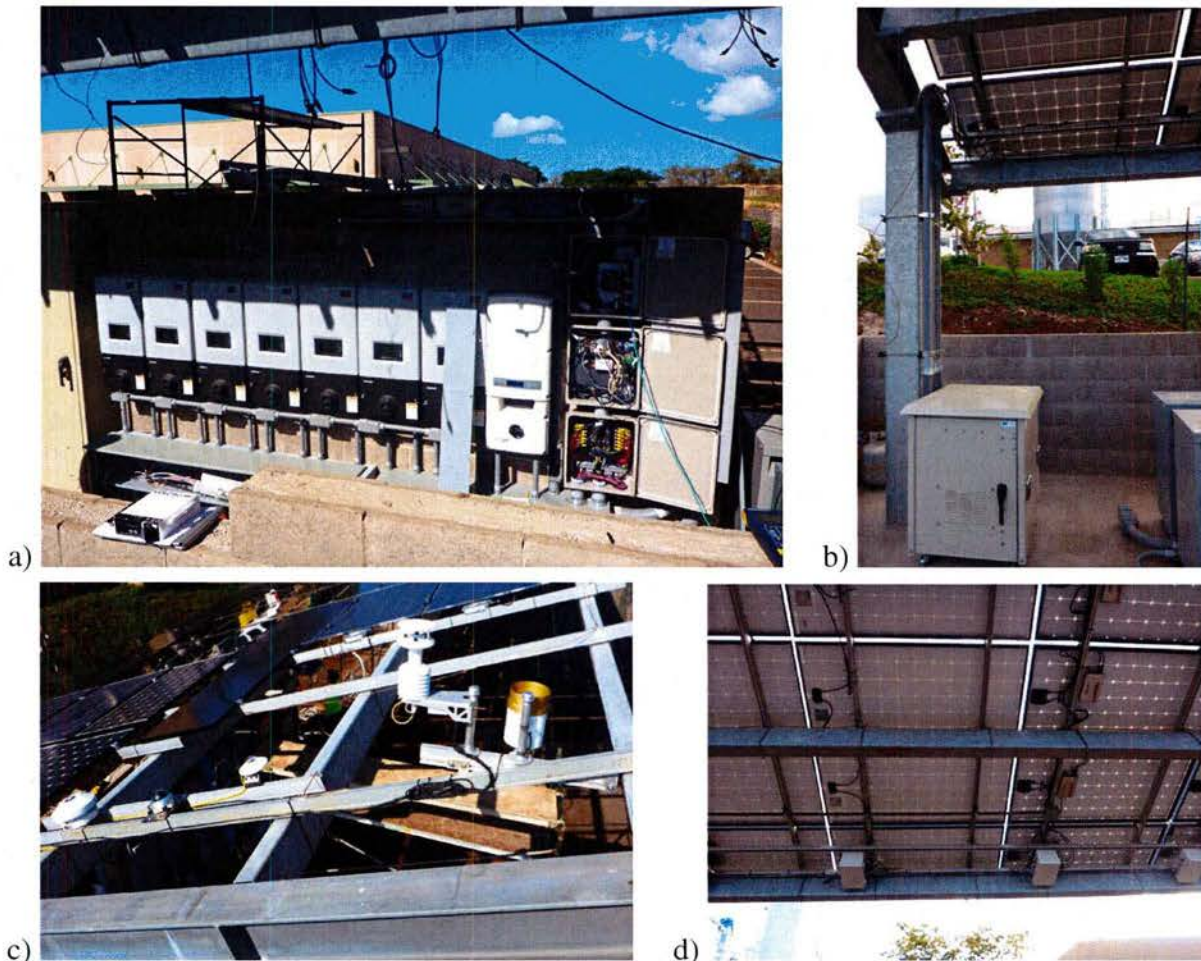
Figure 6.4: The Maui PV test platform during installation, including string inverters, HNEI AC instrumentation, internet connection hardware and DAS controller (a), the IV tracer (b), the weather station and solar sensors (c) and the DC measurement boxes located below the PV modules (d).
