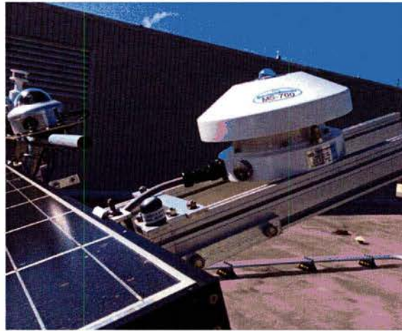
Figure 6.1: Global/diffuse pyranometer on the left and spectroradiometer on the right installed at the Green Holmes Hall Initiative test site (GHHI).
