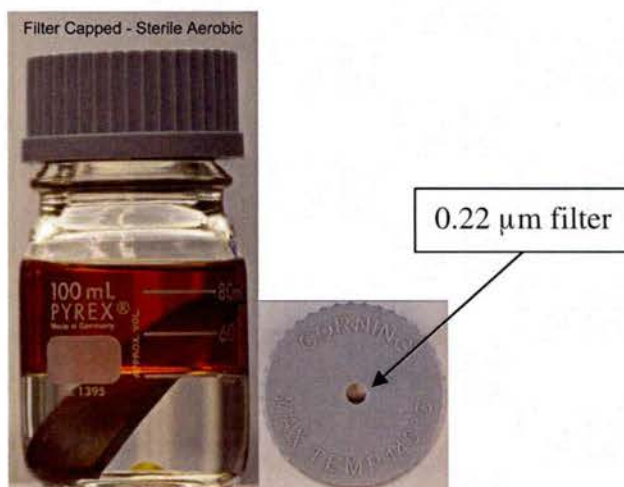
Figure 2.6.1: Fuel-water mixture depicting sterile aerobic environmental setup. Sterile aerobic cap also depicted.
