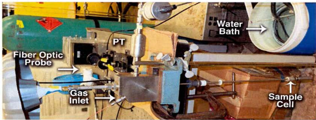
Figure 3.31: Photograph of the fiberoptic probe and gas lines connected to the high pressure cell used to form binary hydrogen hydrates.
