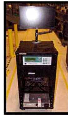
Figure 1.1.8: (left) CO 2 injection syringe with motorized traverse for accurate injections; (right) complete RTD apparatus with computer, vacuum pump, and infrared CO 2 detector.
