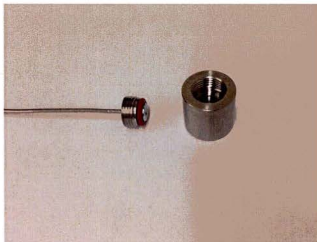
Figure 3.28: Photograph of the MCDSC high pressure sample cell and closure.
