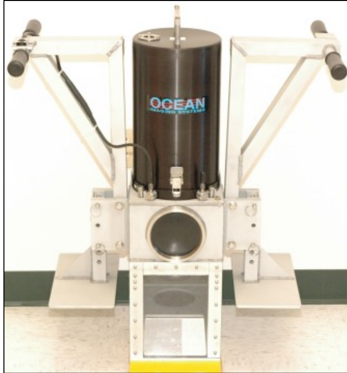
Figure 5-11. The hand-held, diver-deployed sediment profile camera used in Pearl Harbor.
