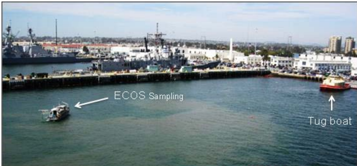
Figure 5-7. Photo of the resuspension event procedure induced by a tug and the ECOS sampling the plume in San Diego Bay.
