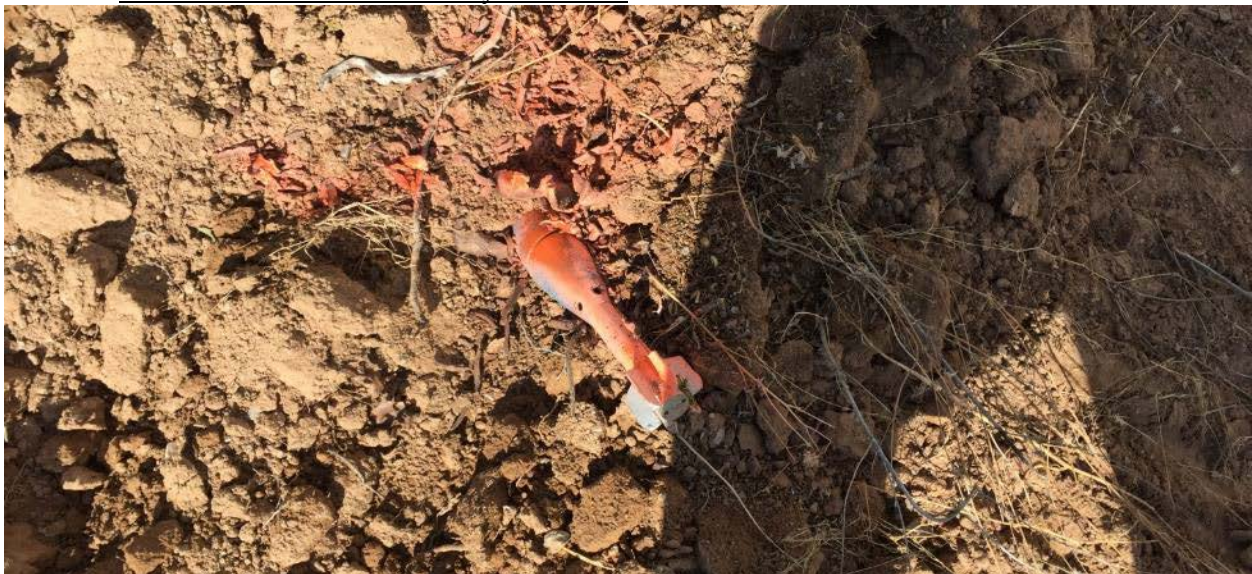
Figure 24: Aluminum rocket not picked up by SAFMSS. The magnet of SAFMSS cannot pick non-ferrous debris.
