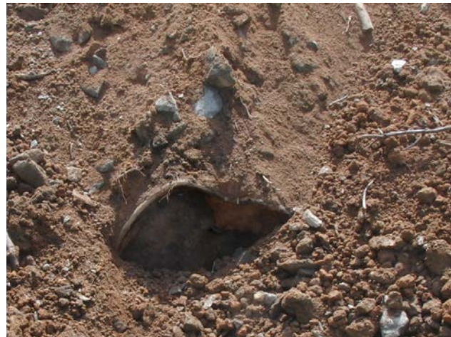
Figure 17: Items not removed by SAFMSS, thin walled and dirt filled objects are problematic due to low ferrous material vs weight with soil.
