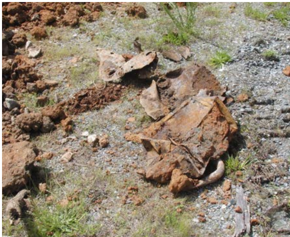
Figure 17: Items not removed by SAFMSS, thin walled and dirt filled objects are problematic due to low ferrous material vs weight with soil.
