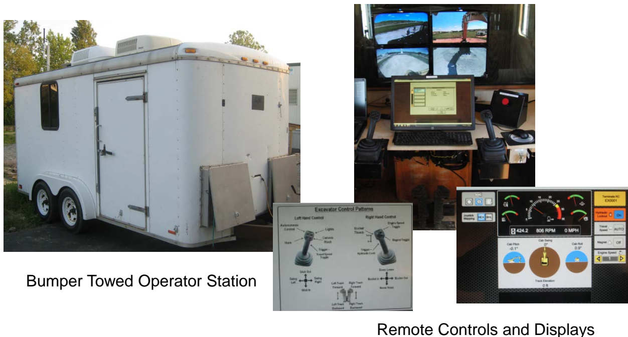
Figure 3: Remote Control Trailer, Controls and Displays
