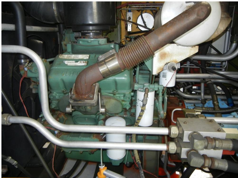
**Figure 10. Detroit Diesel Engine From HT06 Model MJ-2A at MacDill AFB**
