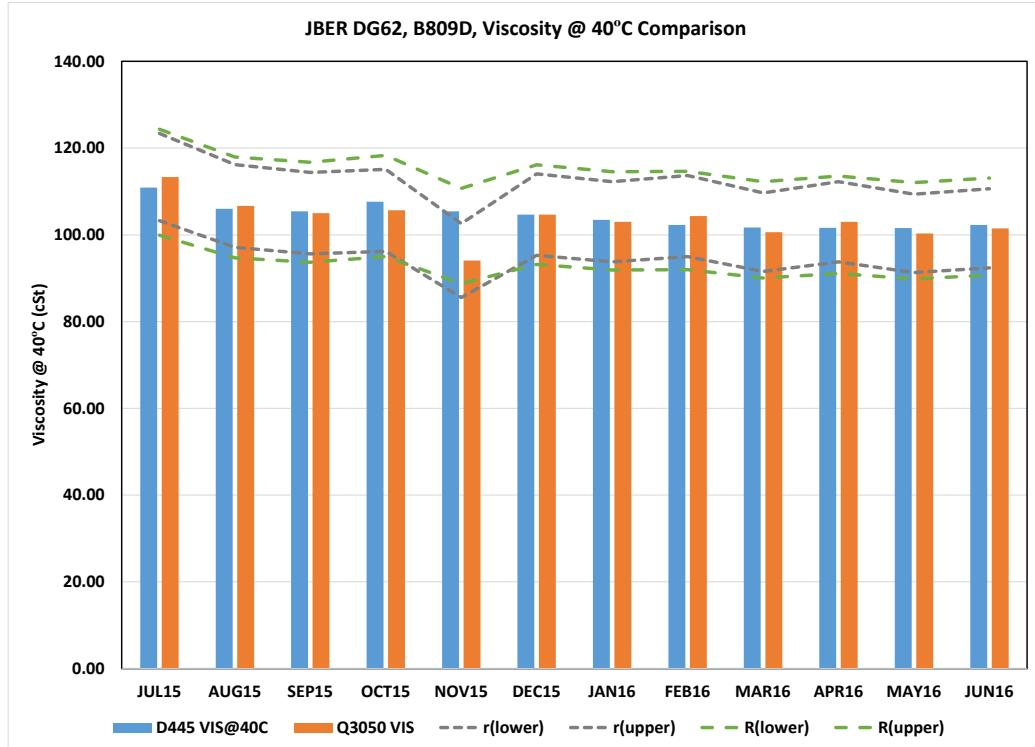
**Figure 27. Comparison of ASTM and Portable Viscosity @ 40 °C for JBER DG62 Asset**
