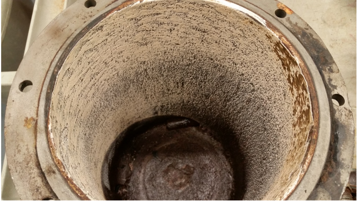
Figure 7. Cast iron vessel after test that had multiple pump failures
