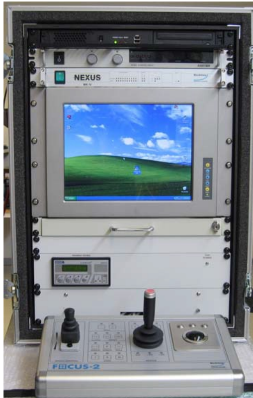
Figure 6. Nexus multiplexer and shipboard control computer and console
