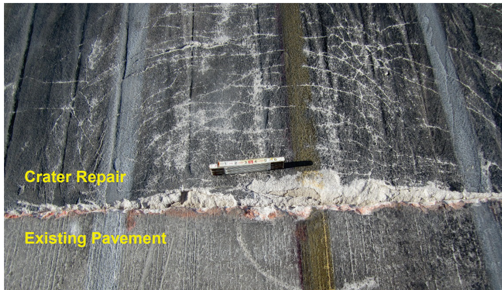
Figure 41. Crater 7, 224 passes, high-severity joint spalling on north edge.
