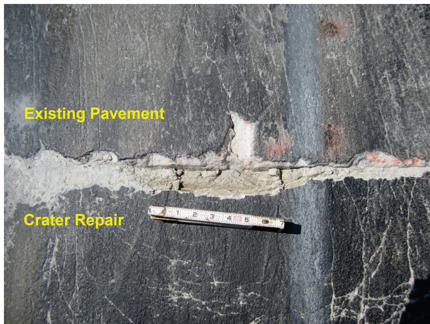
Figure 47. Crater 8, 504 passes, high-severity spalling on south edge.
