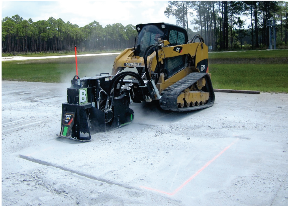
Figure 9. Saw cutting with CTL and wheel saw attachment.
