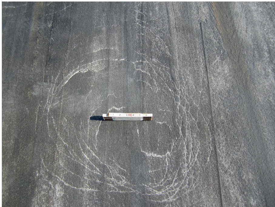
Figure 45. Crater 8, 224 passes, low-severity cracking and depression.
