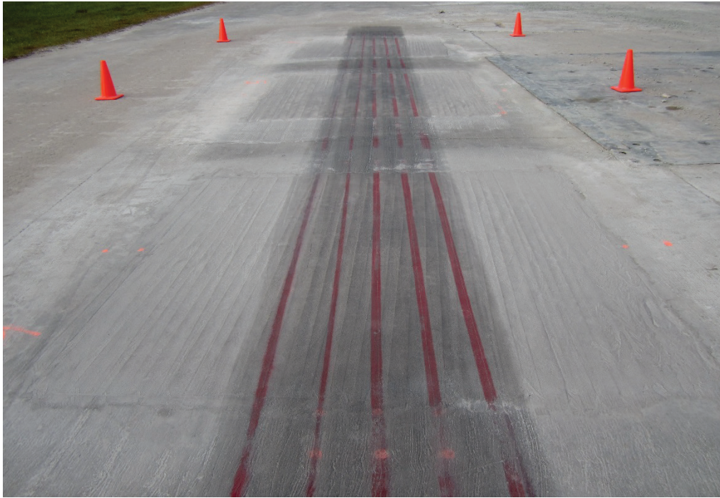
Figure 38. Craters 4, 5, and 6, 512 passes, overall.
