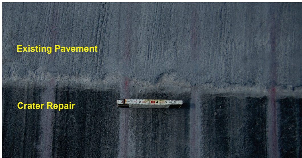
Figure 36. Crater 3, 512 passes, medium joint spalling and depression.
