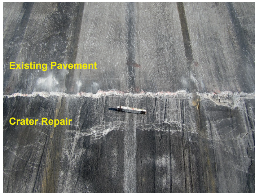
Figure 44. Crater 8, 112 passes, distresses on south edge.
