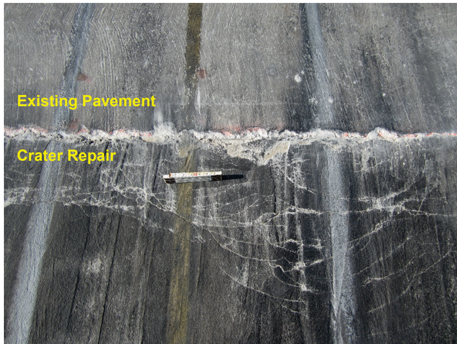
Figure 46. Crater 8, 224 passes, distresses on south edge.
