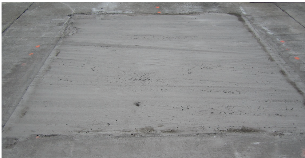
Figure 22. Crater 1 before trafficking.
