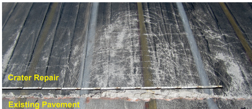
Figure 42. Crater 7, 504 passes, high-severity joint spalling on north edge.
