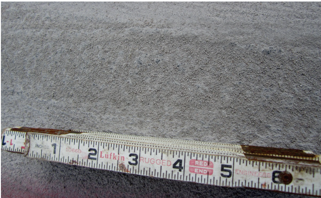
Figure 29. Closeup of small debris on Crater 1 after 112 passes.
