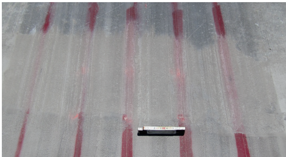
Figure 37. Crater 4, 512 passes, small debris.
