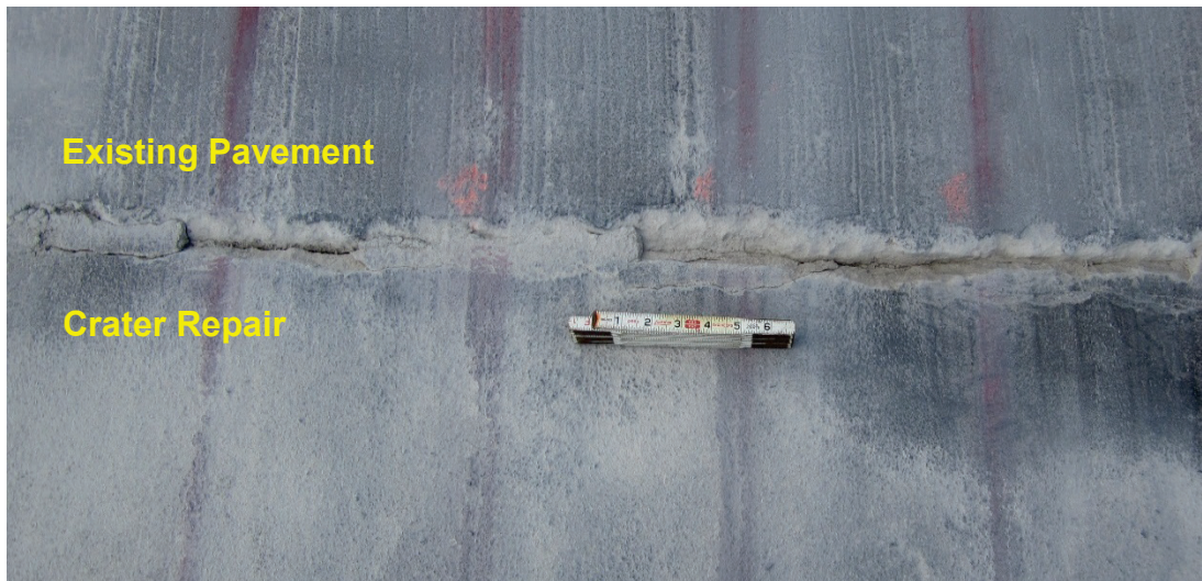
Figure 35. Crater 2, 512 passes, high-severity joint spalling.
