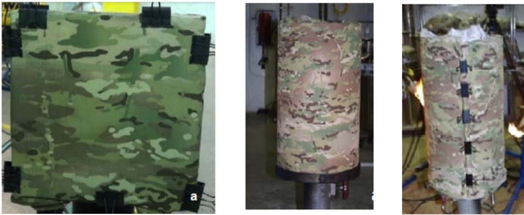
Figure 7. Fabric specimens clamped onto the flat plate and cylindrical test forms
