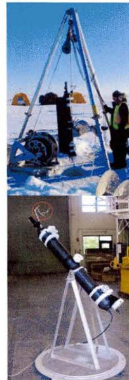
Figure 3. Right. Photograph of an MIZ ITP-V being deployed (top) and in a test jig used to validate sensor orientations (bottom).
