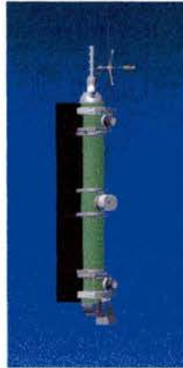
Figure 1. Schematic drawing of the Ice-Tethered Profiler instrument system.
