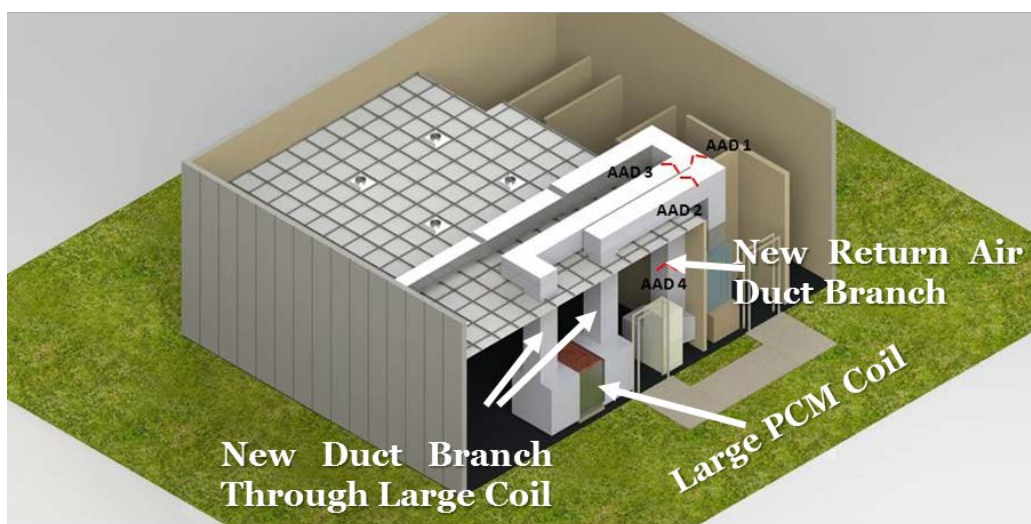
Figure 23: SolidWorks 3D Render of the Demonstration Building Showing Existing Duct Path (Top) and New Duct System After Integrating the Large PCM-Filled Coil (Bottom)
