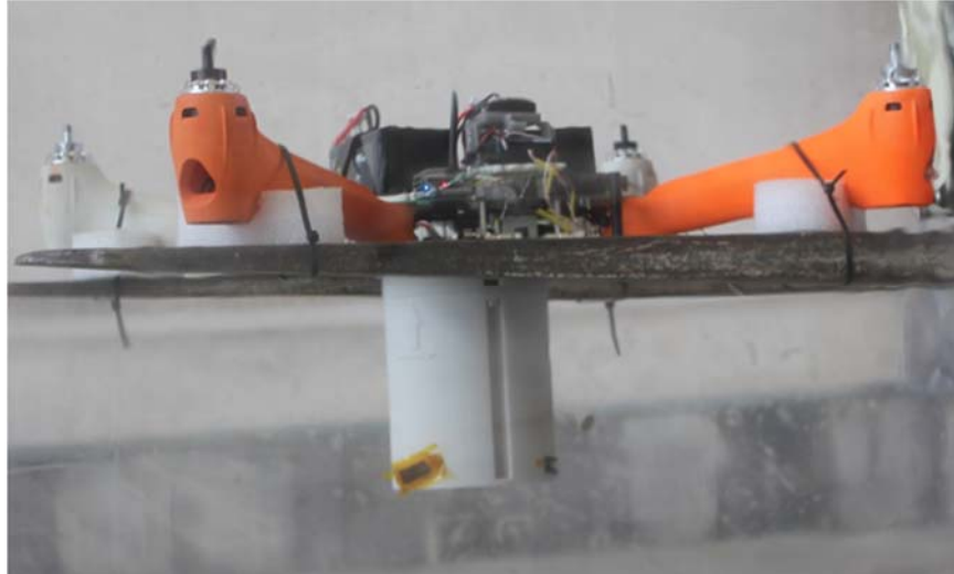
Figure 4. Testing of the ACORNS chemical detection and vapor collection module.
