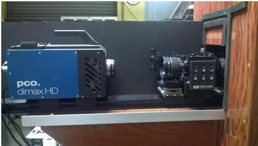
Figure 1. Schlieren optical system showing the pco.dimax HD camera and the visible section of the lens assembly.
