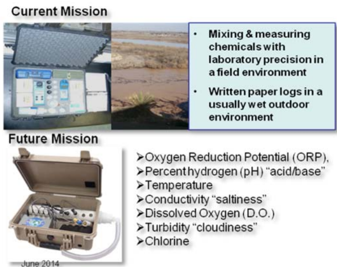
Figure 6: Current Manual Water Monitoring Process (Top) and WATERMON (Lower Left)
