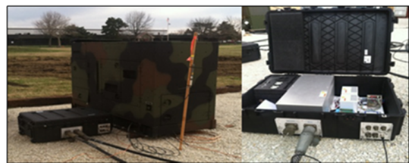
Figure 11: DIACAP Approved Wireless Metering Solution Interfacing with a Generator Set
