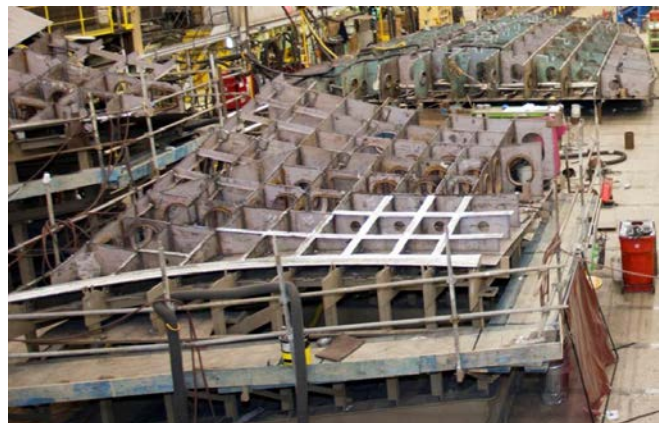
Robotic welding of innerbottoms and side shell assemblies will improve productivity and reduce costs of DDG 51 construction. BIW photo
