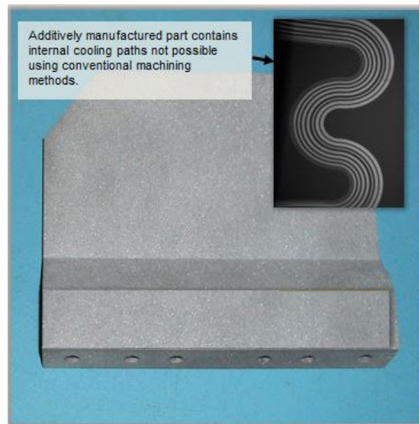
Maturing additive manufacturing technologies to fabricate metal electronics chassis on Navy platforms will reduce cost and lead time. Raytheon image
