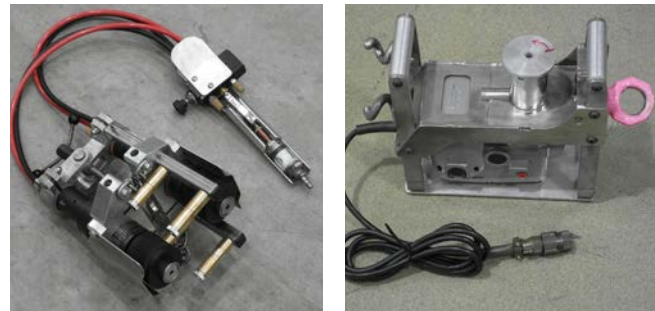
Tools developed under the Mechanized Cable Pulling project will reduce labor as well as health and safety issues associated with shipboard cable pulling. Pictured are the capstan (left) and dual roller (right) tools. NMC photos
