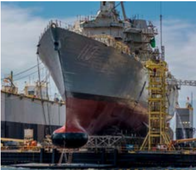
New tools and technologies will reduce time, labor, and rework associated with sonar dome fabrication. Ingalls photo
