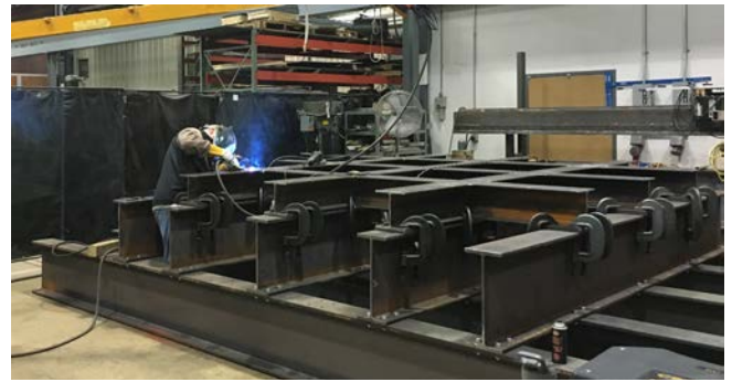
A new joint detail that enables Self-Locating/Self-Fixtured (SLSF) deck construction for OR and VPM deck flats will reduce labor hours and costs. Electric Boat photo
