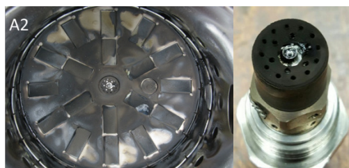
Figure 6. Combustor Liner and Fuel Nozzle after 5 Hours of Operation Using a 5% Skydrol/F-24 Fuel
