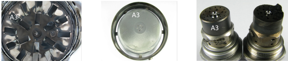
Figure 15. Combustion Liner, First Stage Heat Shield, and Fuel Nozzle after 25 Hours of Operation Using a 1% Skydrol 5 with F-24 for Fuel
