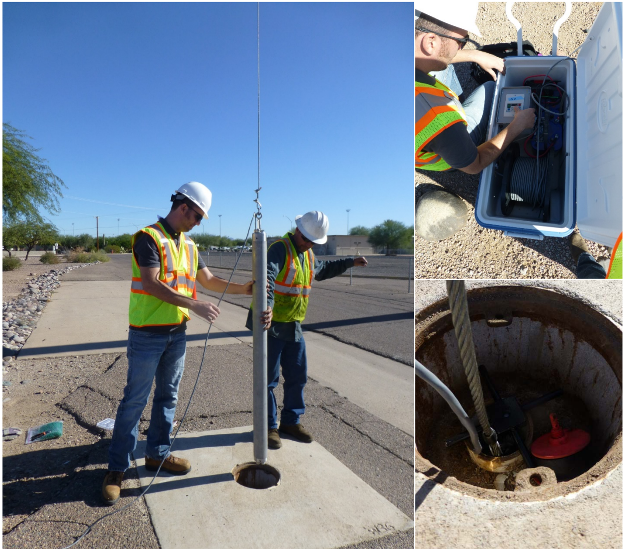
Figure 5-18. Deployment of the IS2 sampler into W36 at the former Williams AFB, November 2013. Clockwise from left: 1) insertion of the sampler by crane, 2) the surface package being programmed, and 3) the deployment hanger on the well head.
