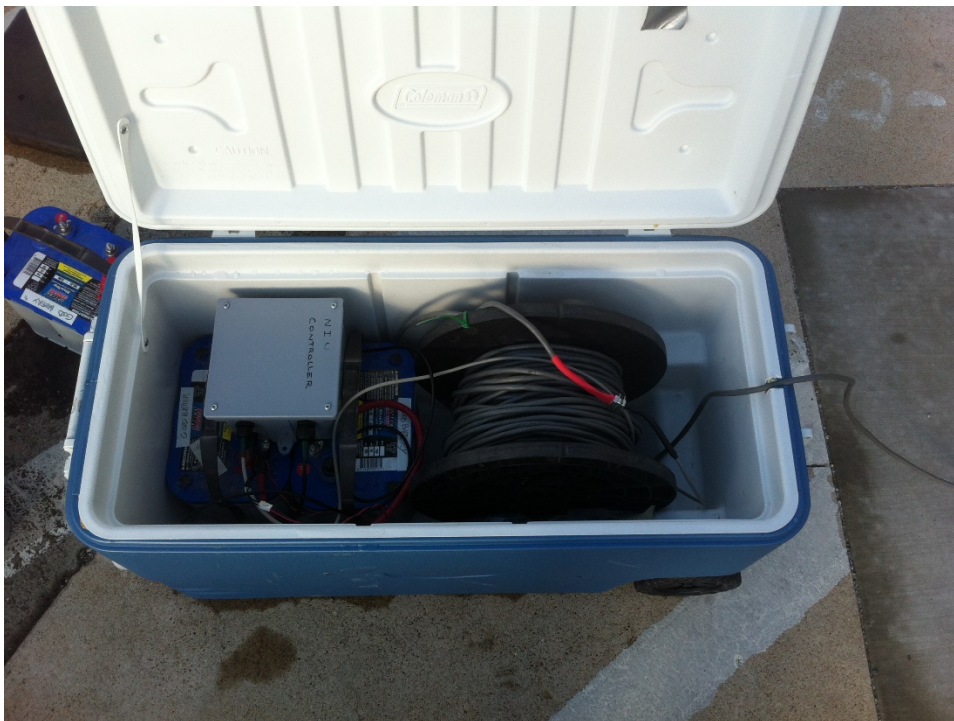
Figure 5-14. Field-prepared IS2 surface package for reciprocating syringe pump.
