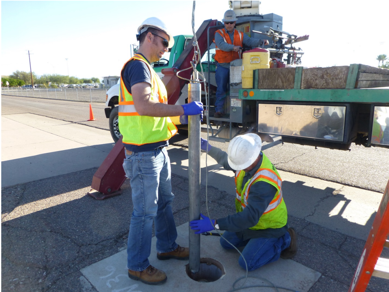
Figure 5-17. Installation and deinstallation of an IS2 sampler with a crane.
