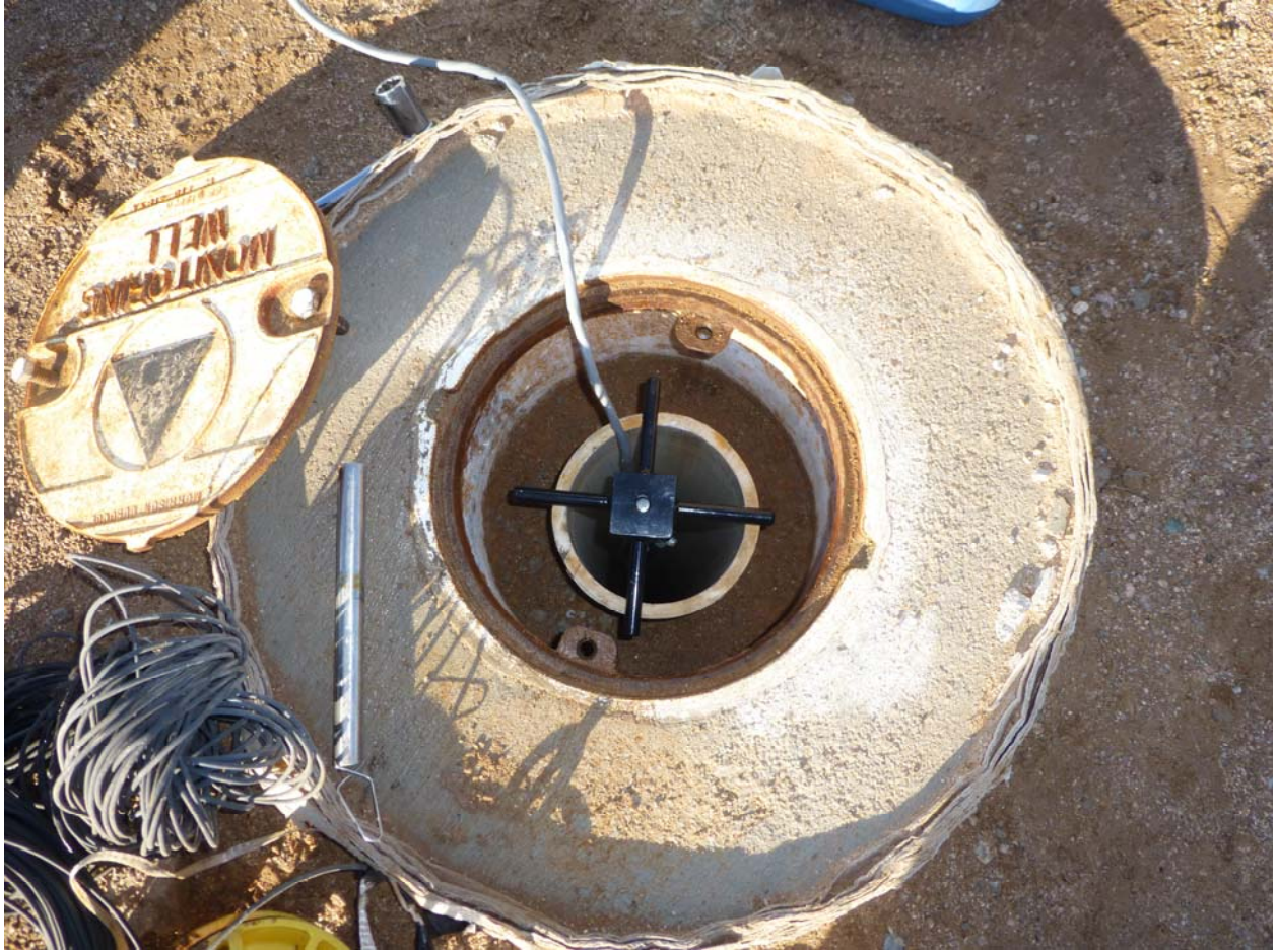
Figure 5-5. IS2 Sampler deployed in a monitoring well at the perchlorate site in 2012.
