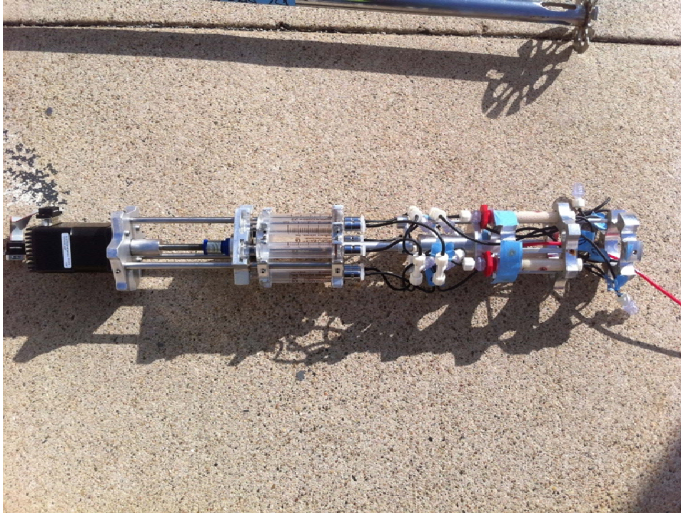
Figure 5-12. Field-prepared IS2 sampler with reciprocating syringe pump.
