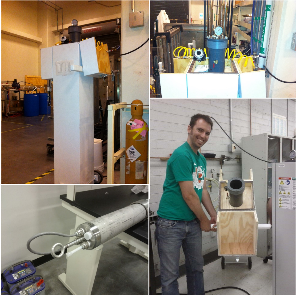
Figure 2-5. Pressure chamber for submersible testing. Clockwise from upper left: 1) pressure chamber installed in laboratory, 2) pressure regulator and gauge, 3) unit has wheels and handle for relocation, 4) an IS2 sampler shell with dummy fittings for pressure testing.
