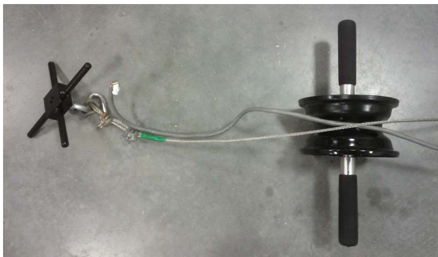
Figure 5-16. Hanger, steel cable, electrical cable, and cable management pulley for deployment of the IS2 sampler.
