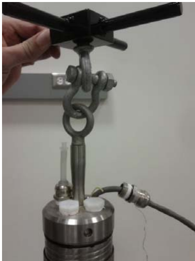
Figure 5-15. Hanger used to secure the sampler in a well.
