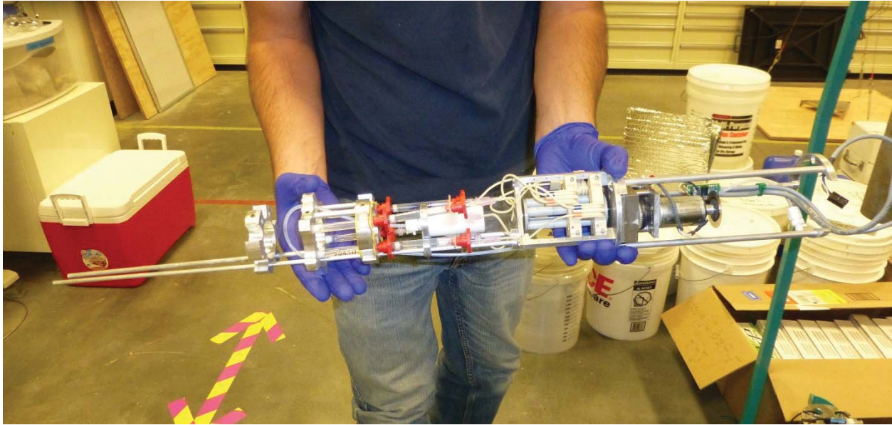
Figure 3. Field-prepared IS2 sampler with peristaltic pump. From right to left, the unit comprises a peristaltic pump and an array of cartridges for solid phase extraction.
