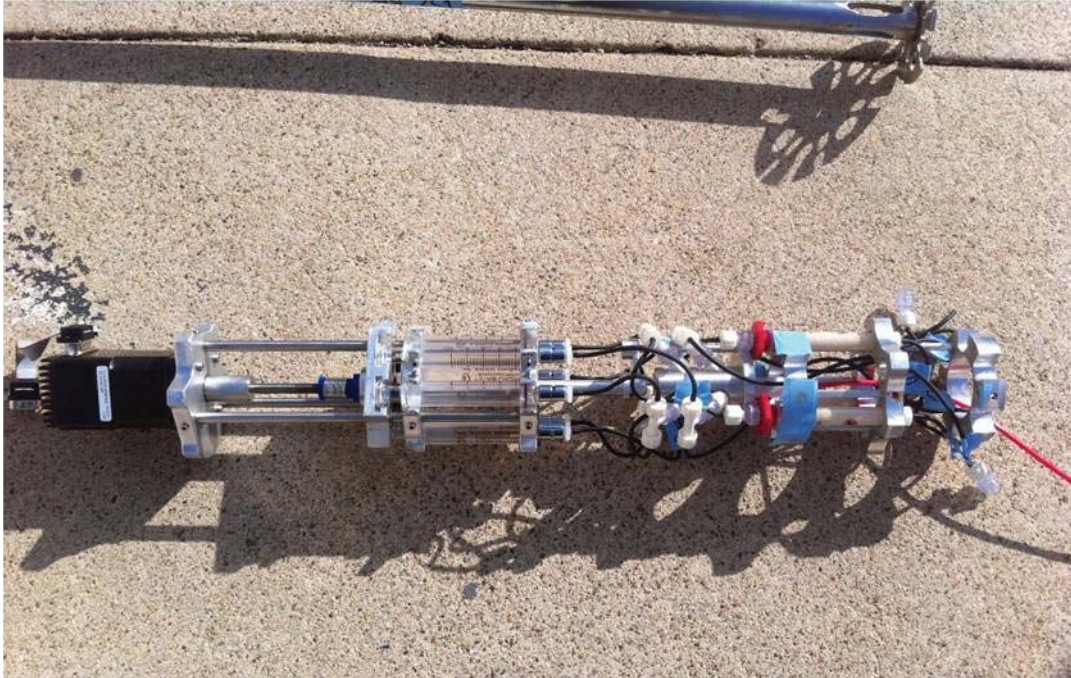
Figure 14. Field-prepared IS2 sampler with reciprocating syringe pump.
