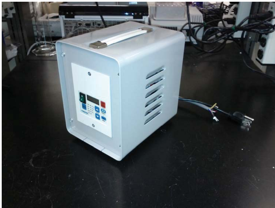
Figure 10. IS2 peristaltic pump control unit.
