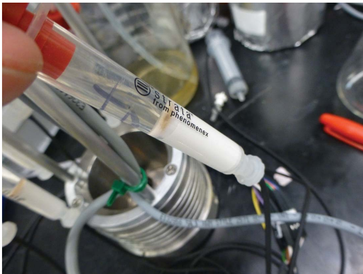
Figure 23. Accumulation of surface water sediments upon the frit of an SPE cartridge.
