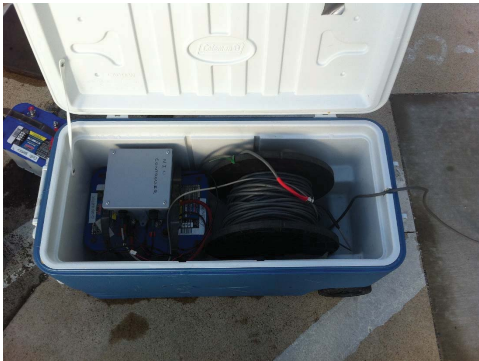
Figure 16. Field-prepared IS2 surface package for reciprocating syringe pump.
