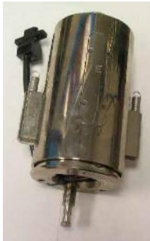
Figure 3. Vertical Engage Scanner. This makes work easier and faster. It is faster and more secure to adjust for differences in sample thickness. With a top view optical microscope, it can target a specific area and engage the probe tip at that spot.
