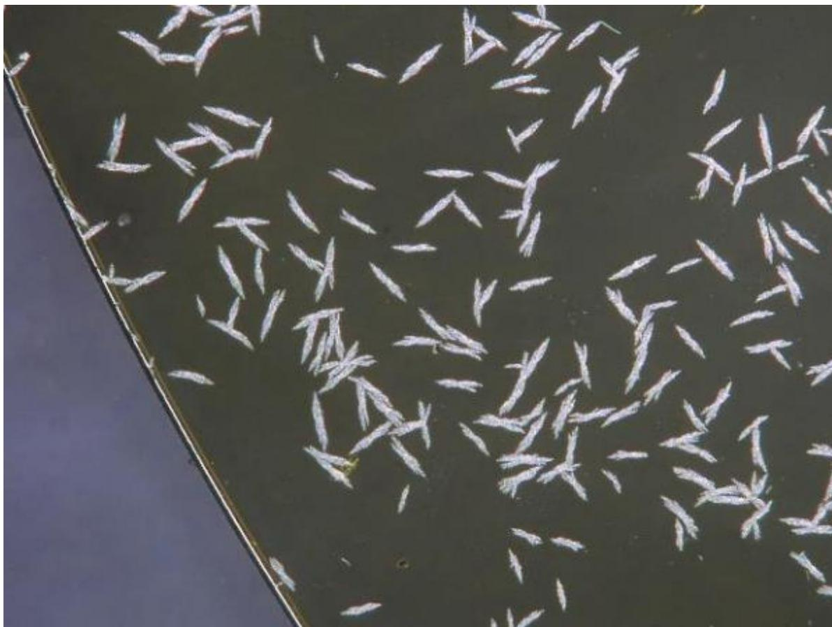
Figure 3. Optical Image of MoS<sub>2</sub> on a sapphire substrate. The ‘scratches’ on the sample is actually excess sulfur that coalesced on the substrate during the final stages of the growth process. These were burned off during XPS without damaging the sample.
