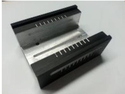
Figure 7: Four point bending fixture
