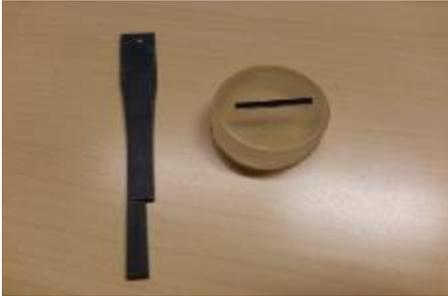
Figure 5: Specimen after cut (left) mounted and polished sample (right)
