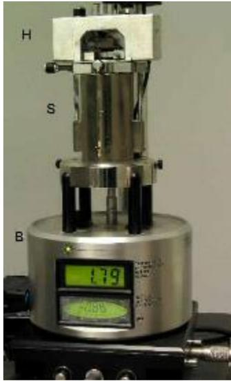
Figure 2. The MultiMode AFM consists of a Base (B), a Scanner (S), and an optical head (H).
