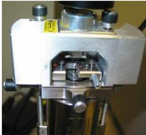
Figure 5. MultiMode AFM with sample in place, ready to scan.
