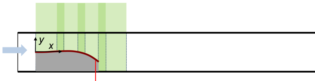
Figure III.3-3. The PIV field of view of the flow in the x - y plane of the 25 mm wide channel z = H/2 over the reed and downstream of its trailing edge. Multiple streamwise positions of the laser sheet are shown with some overlap. The laser beam of the range finder is also shown for reference within the reed's shadow (shown in gray).
