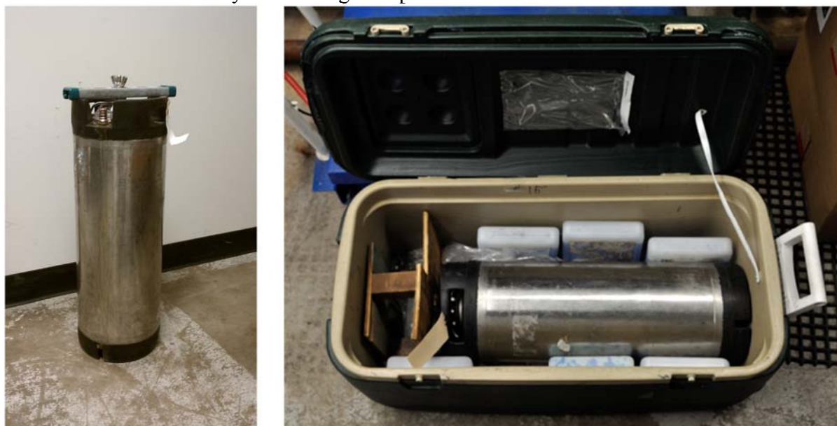
Figure 5.22. Photographs of 20-L soda keg used for culture starvation and shipping. The kegs were packed in ice prior to overnight shipment to the field in coolers.
