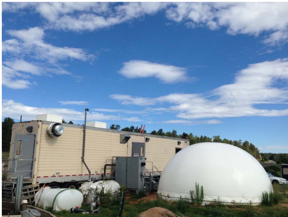
Figure 22. Biogas holder adjacent to the demonstration trailer.
