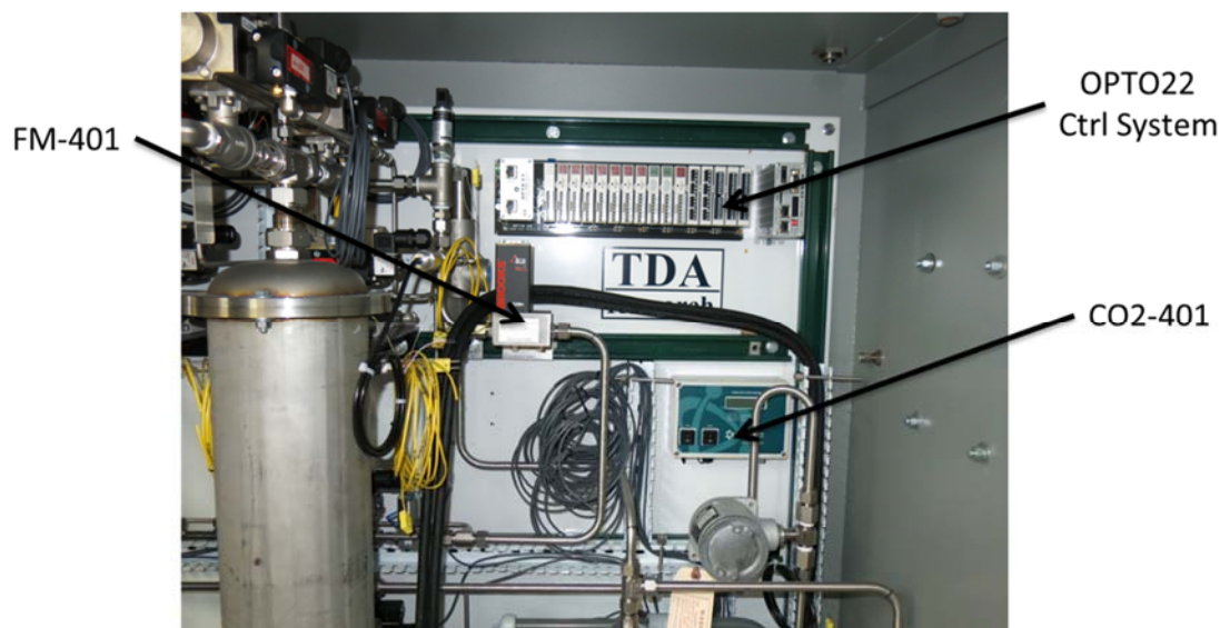
Figure 23. Picture of the pilot scale unit showing the product methane flowmeter (FM-401), product CO 2 analyzer (CO2-401), and OPTO22 Control System.
