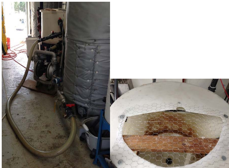
Figure 19. Feed tank, diaphragm pump, transfer hose, and digester with close-up of chicken wire screen on feed tank lid.
