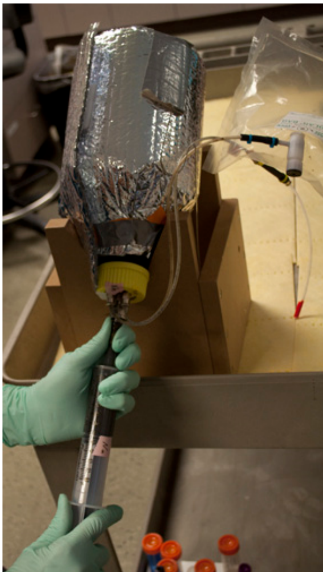
Figure 4-4 Sampling of 2L,Semi-Continuous Reactor
