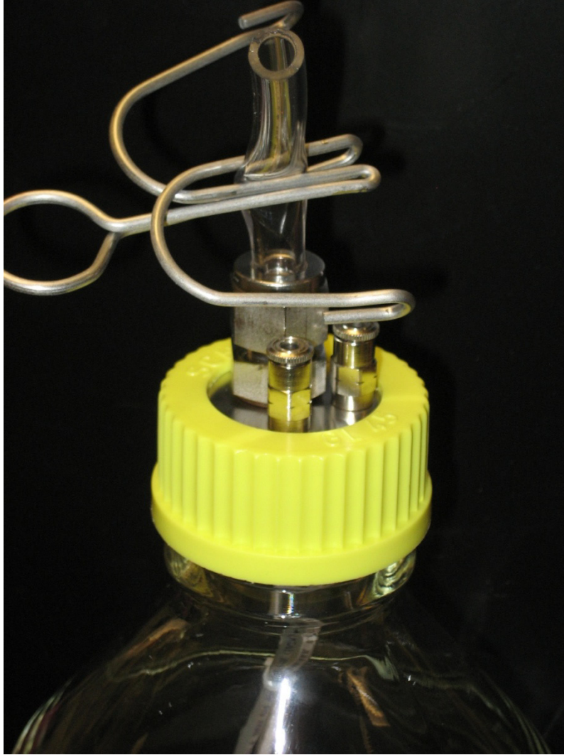
Figure 4-3 Configuration of 2L Semi-Continuous Reactor Bottle
