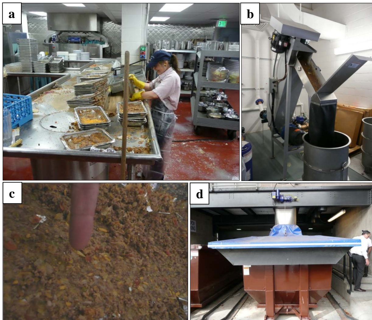
Figure 25. Food waste at Mitchell Hall was manually scraped into recirculating sluice water which was then ground in a pulper/shredder (a). The slurry gravity-drained down one floor into dewatering equipment (b). The dewatered and ground food waste (c) then dropped into a roll off container (d) on the floor below where it was sent to a landfill. Food waste was collected in 5-gallon buckets from the dewatering system (c).
