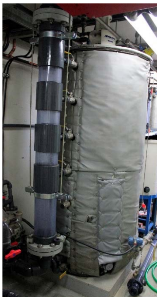
Figure 18. Insulated digester tank and foam pot.
