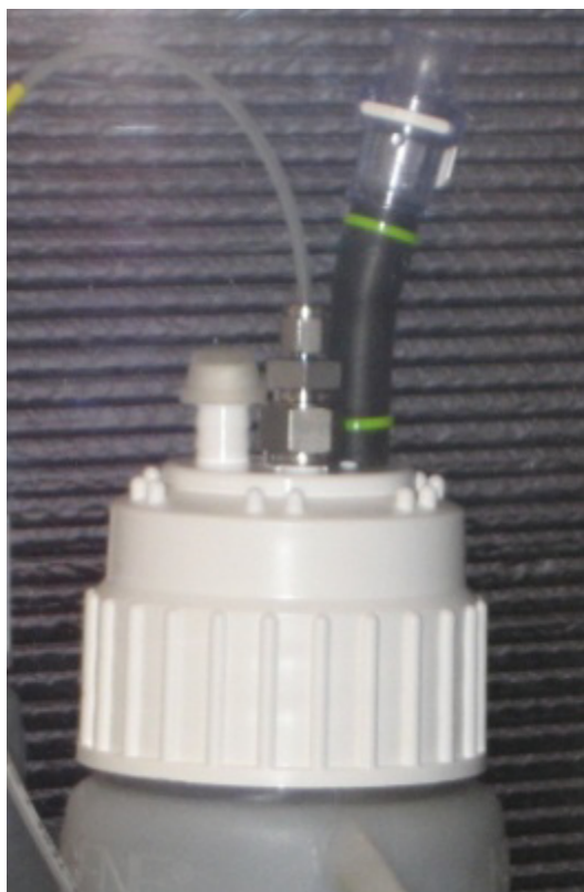
Figure 4-2 Carboy Cap with Headplate Connections
