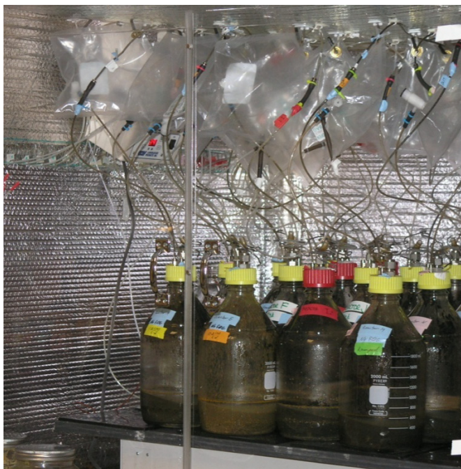
Figure 4-5 Reactors on Shaking Table in Incubator
