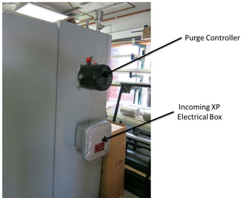
Figure 24. Picture of the pilot scale unit showing the Type X purge controller and the incoming XP electrical box.
