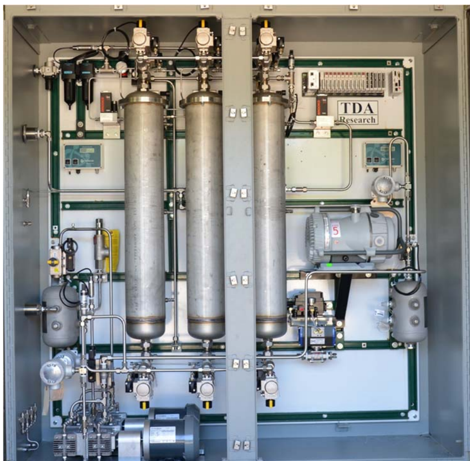
Figure 20. Picture of the pilot scale CO 2 and H 2 O removal unit.
