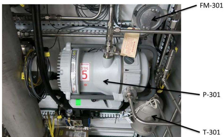
Figure 21. Picture of the pilot scale unit showing the blowdown gas flowmeter (FM-301), water knockout (T-301) and the vacuum pump (P-301).
