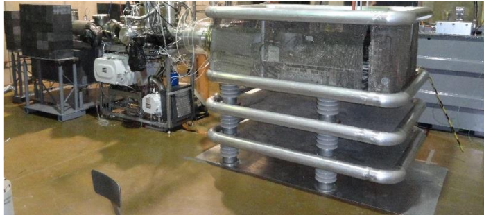
Figure 7 PNL high yield, long lifetime neutron generator
