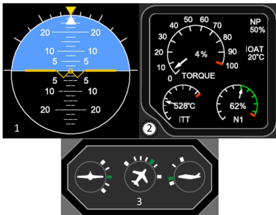
Figure 8.9.5.1-1. Pitch (1), Bank (1), Power (2), and Trim (3) Instrumentation.
