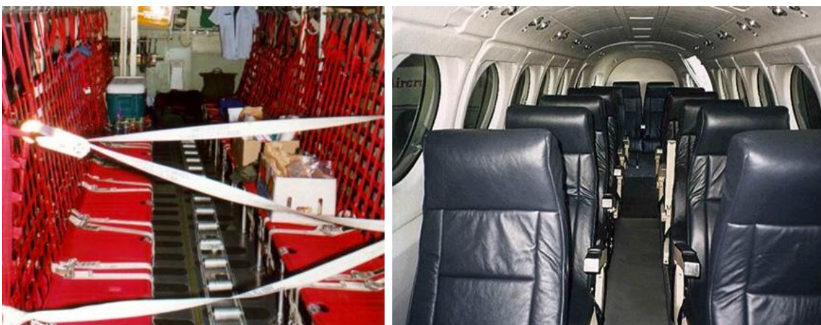
Figure 7.6.5-1. C-130 Web Seating with Aluminum Supports (Left) and High-Density Foam Seats with Leather Exterior (Right)
