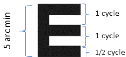
Figure 1.4.5.1-3. Each Snellen “E” Contains 2.5 Cycles
