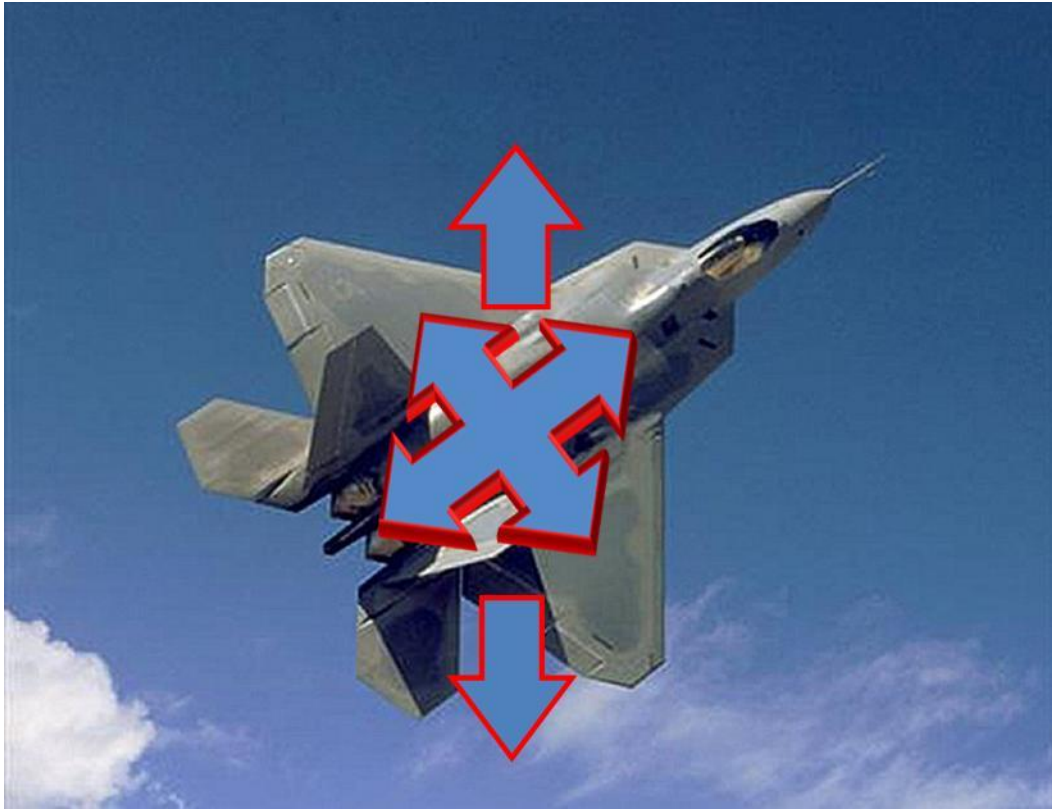
Figure 7.2.2-1. Vibration Axes during Combat Maneuvering
