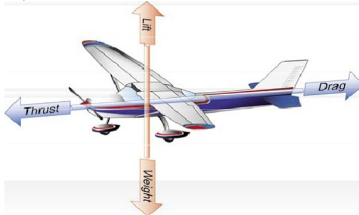
Figure 8.9.3-1. Aerodynamic Forces Acting on and Aircraft (FAA, 2016)
