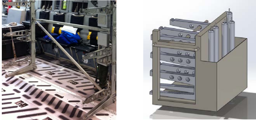
Figure 6. Stanchion rack concept for the C-17.
