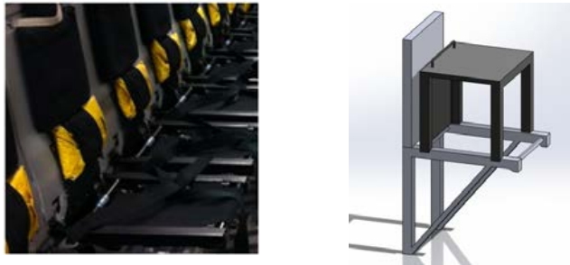
Figure 7. Step stool concept for hanging lines during C-17 configuration.
