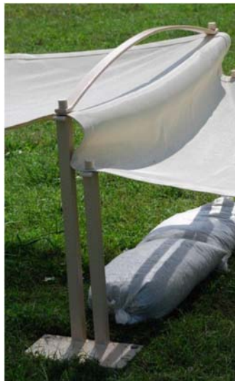
Figure A-11. Crawls. a) Layout of the Crawls station showing the location of the sandbags and the height change at the transition point. b) Close-up of the height transition poles.
