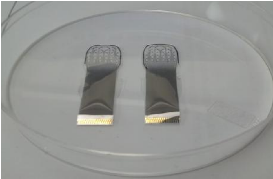
Figure 8. Two \mu ECoG arrays released from a silicon carrier wafer.
