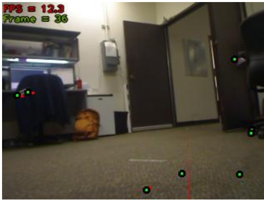
Fig. 13. Lack of reliable feature points (green) to track to calculate accurate camera motion. Red bar indicates displacement of the tracked features from the previous frame.
