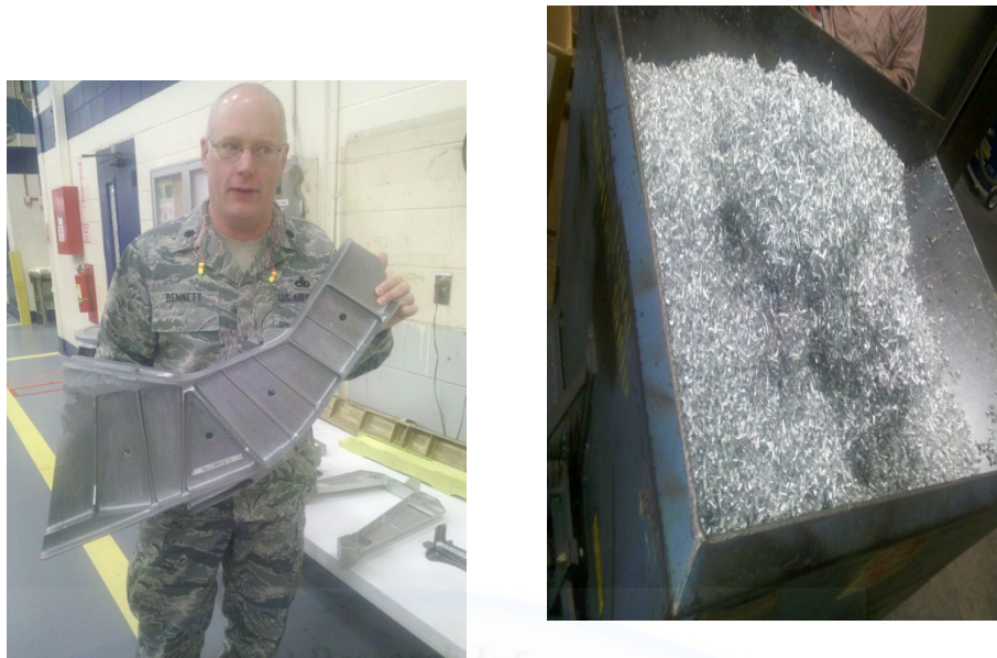
Figure 1: C-5 End Fitting and Machine Waste
