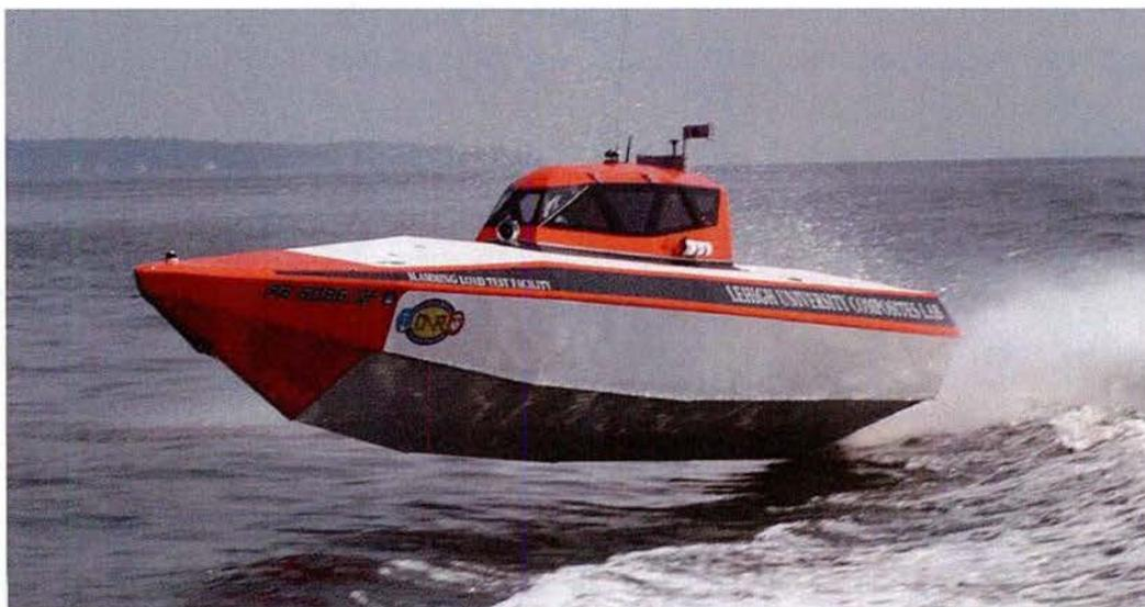
**Fig. 1.** The Numerette in operation. The boat was designed for 23 G vertical acceleration.
