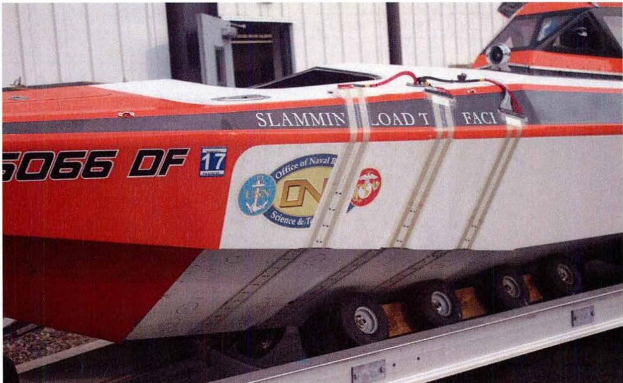
**Fig. 9.** Externally mounted film pressure sensors.
