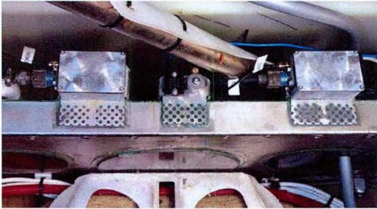
**Fig. 4.** Two INS modules, a triaxial piezoelectric accelerometer and a single-axis MEMS accelerometer, mounted on the transverse bulkhead #2 just in front of the engine.
