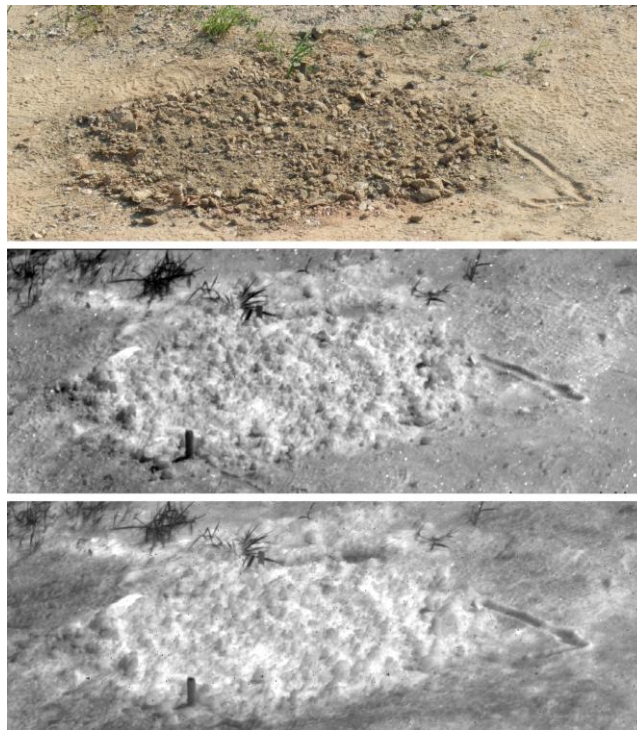
Figure 6. Soil imaged immediately after disturbance. From top to bottom: visible, 3.8 - 4.2 \mu\text{m} , 4.5 - 5 \mu\text{m} . High phase (viewing into sun), providing significant shadows for increased salience in visible and at the shorter mid-IR band. Note the generally softer appearance of the longer band IR image compared to the shorter wavelength IR image, specifically the foot prints in the upper right are apparent in the top two images but less salient in the bottom. Scale: the images are foreshortened and are ~ 3 feet in each direction.
