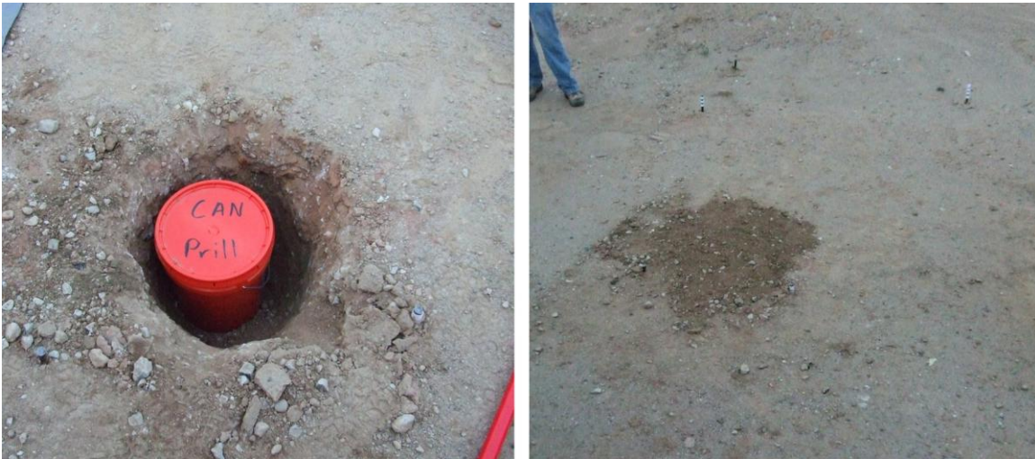
Figure 1 Day 1. 07/28/10. Example buried object and surrounding undisturbed soil. Visible salience enhanced due to higher moisture content of the recently subsurface soil.
