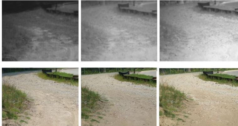
Figure 5. Illumination geometry strongly affects the saliency of a disturbed gravel road. Illumination trends left-to-right, from high phase (looking into the sun), high sun, to low phase (sun behind observer). Higher phase observations have more shadows and enhance surface roughness, especially in absence of other sources of brightness differences.
