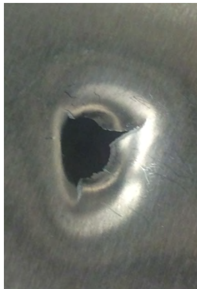
(b) Isometric view of projectile shot plate
