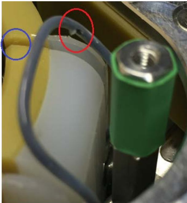
Figure 79. HCT antenna hold down coating degradation
