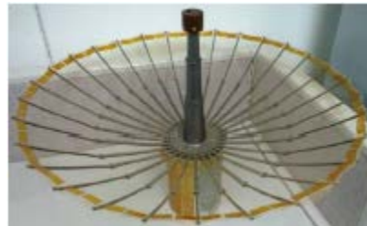
Figure 11. SERC and NASA/JPL parabolic antenna prototype [28]
