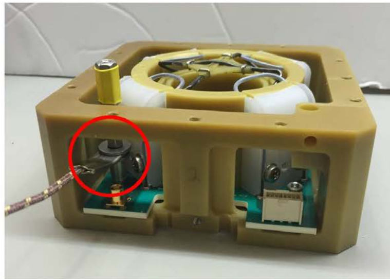
Figure 2. HCT Antenna Thermocouple Placement, Side View
