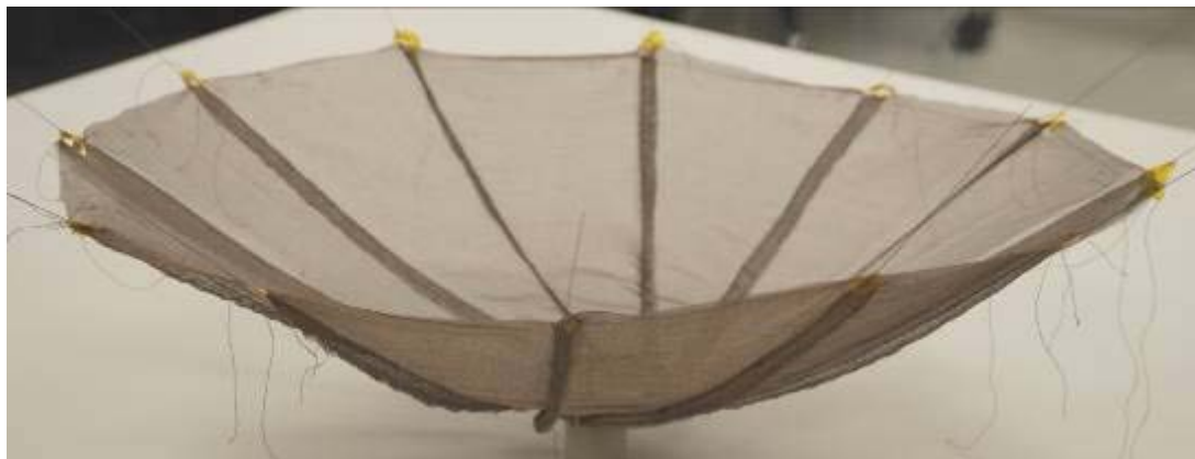
Figure 16. Boeing Phantom Works deployable CubeSat mesh antenna prototype [30]
