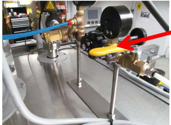
Nitrogen valve on top of chamber
