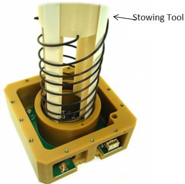
Figure 31. HCT QHA stowing tool [45]
