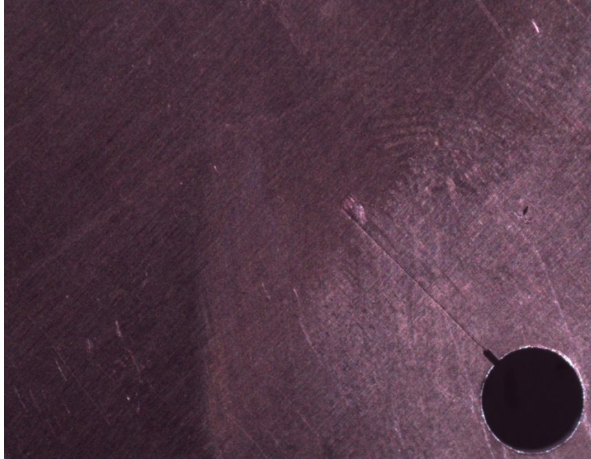
Figure 57: Crack before failure while running R=0.7 experiment in air environment.
