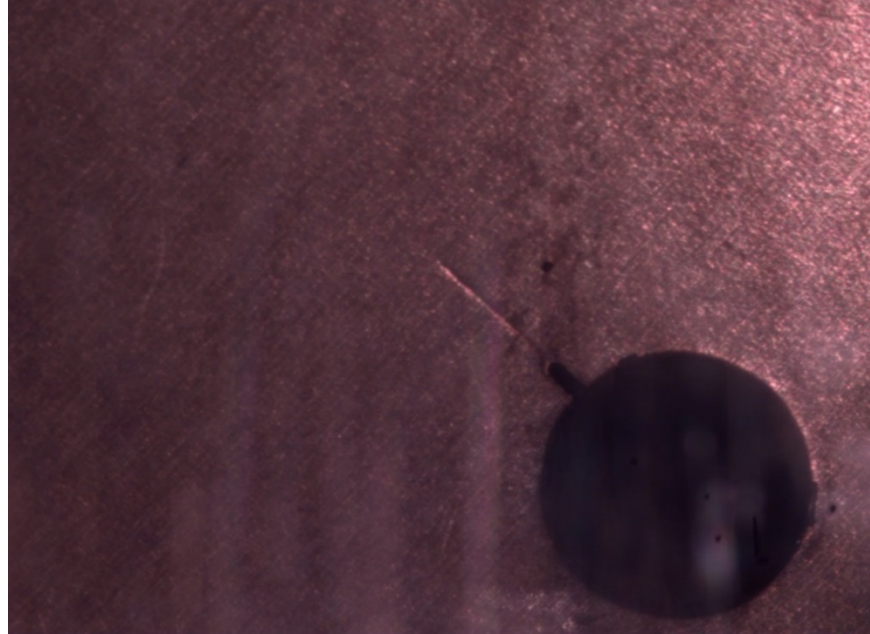
Figure 59: 3.44 mm length crack after applied 92,000 fatigue cycles in saltwater environment at stress ratio of 0.7.
