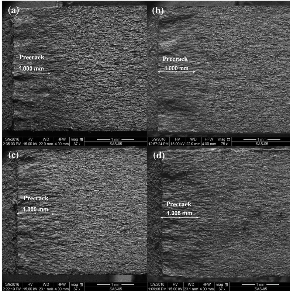
Figure C.9: SEM Images of Fracture Surfaces for Different Biaxial Cases in Saltwater Environment: (a) biaxial ( $\lambda= 0.5$ ), (b) uniaxial ( $\lambda= 0$ ), (c) biaxial ( $\lambda= -0.5$ ), (d) biaxial ( $\lambda= -1$ ).
