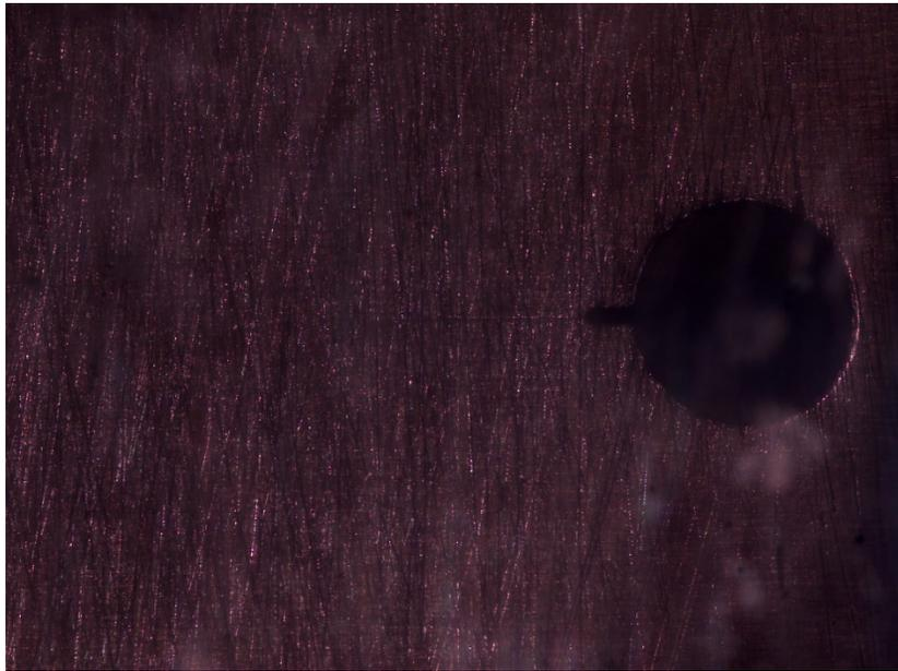
Figure B.4: Crack Shape for  $\lambda=0.5$  at 120,000 Cycles in Saltwater Environment.
