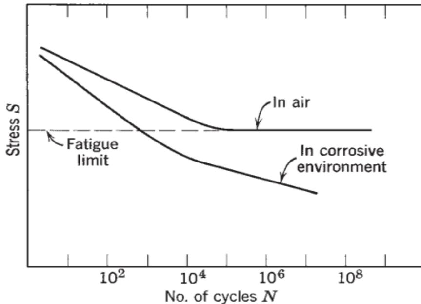
Figure 2.3: The Effect of Environment on the Fatigue Limit of a Material [42].
