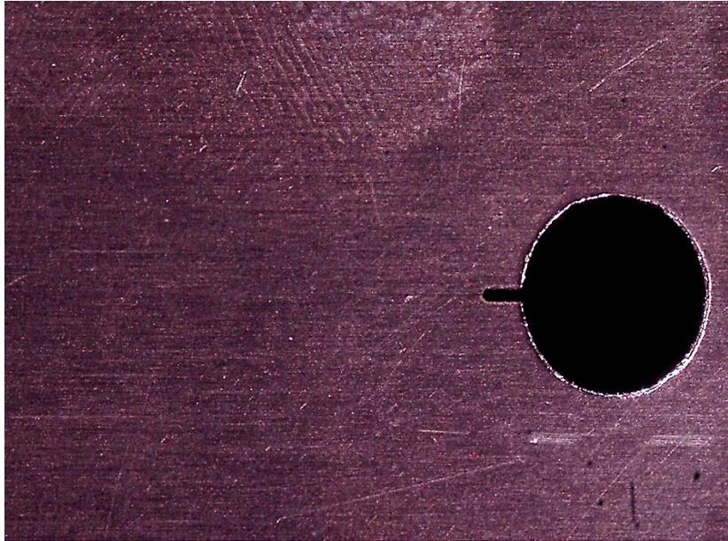
Figure B.1: Crack Shape for  $\lambda=0$  at 220,000 Cycles in Air Environment.
