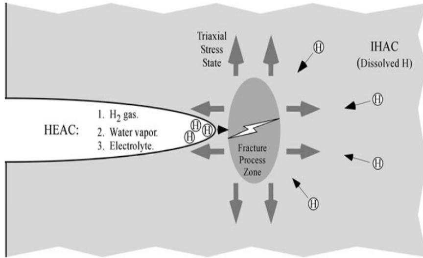
Figure 2.2: Mechanism of Corrosion Due to Hydrogen Embrittlement [5].
