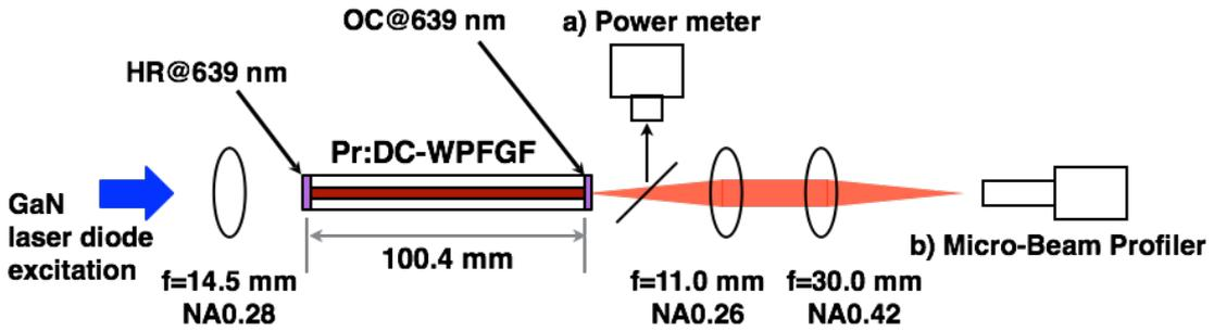
**Fig. 5** Experimental setup for visible fiber laser oscillator in Pr:DC-WPFGF. a) Measurement for input-output characteristics on CW red laser oscillation, and route b) Measurement for beam-quality factor.
