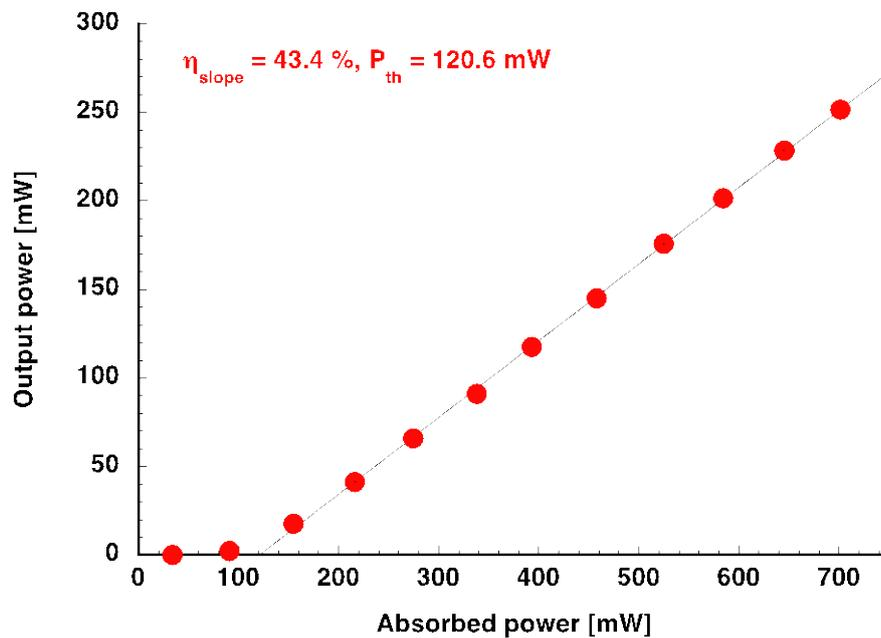
Fig. 11 *Input-output characteristics of CW red laser oscillation.*
