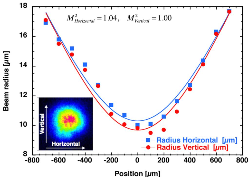
Fig. 13 Beam-quality factor measurement on Pr:DC-WPFGF laser.
