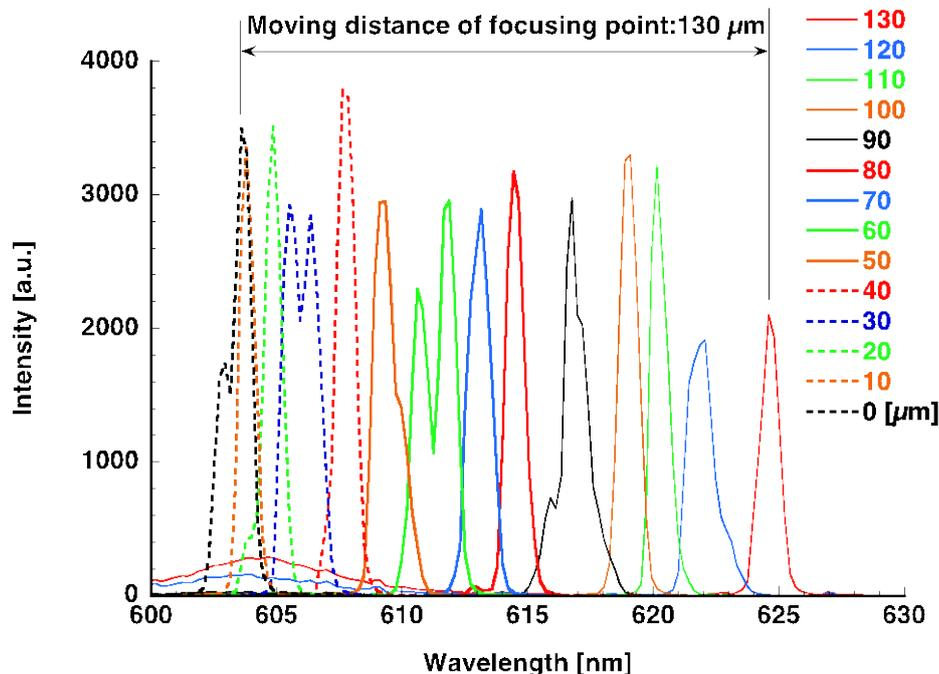
**Fig.10** Experimental result of the presented simple and compact tunable laser.
