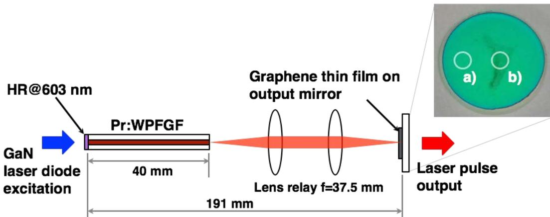
**Fig. 2** Experimental setup for Pr:WPF GF visible pulse laser oscillator and a photograph of transcribed graphene thin film on a dielectric cavity output mirror. a) Focus spot for CW laser operation and b) Focus spot for pulse laser operation.
