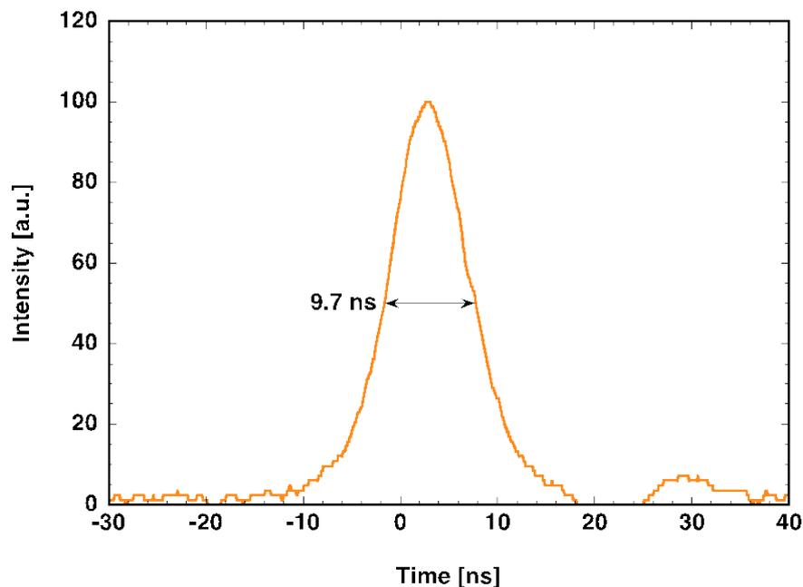
**Fig. 9** Pulse laser generation in Pr:WPF GF.
