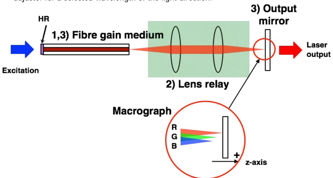
**Fig. 3** Configuration of the presented simple and compact tunable laser. 1)-3) represent and explain the three elements in the text.
