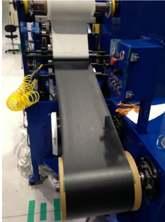
Figure 23: 145 gsm aerospace prepreg prepared from 10wt% MWCNT impregnation film
