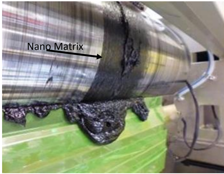
Figure 20: 15.0% MWCNT aerospace epoxy loaded onto an industrial roll coater
