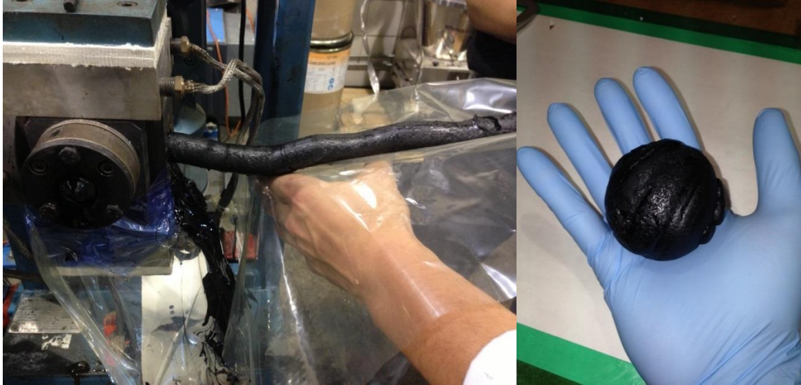
Figure 19: 15% MWCNT epoxy nanocomposite prepolymer (30 LBS/h; 90 sec residence time)
